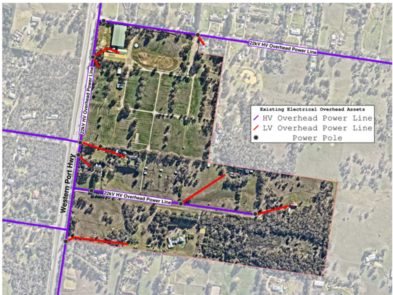
Figure 15 Existing Electrical Overhead Assets (Adapted from BYDA and United Energy Asset Map, 2025)
