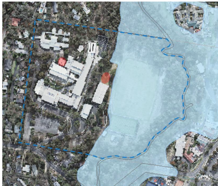
Figure 27 Extent of 1% Annual Exceedance Probability (1 in 100-year flood) and LSIO - development areas highlighted in red
