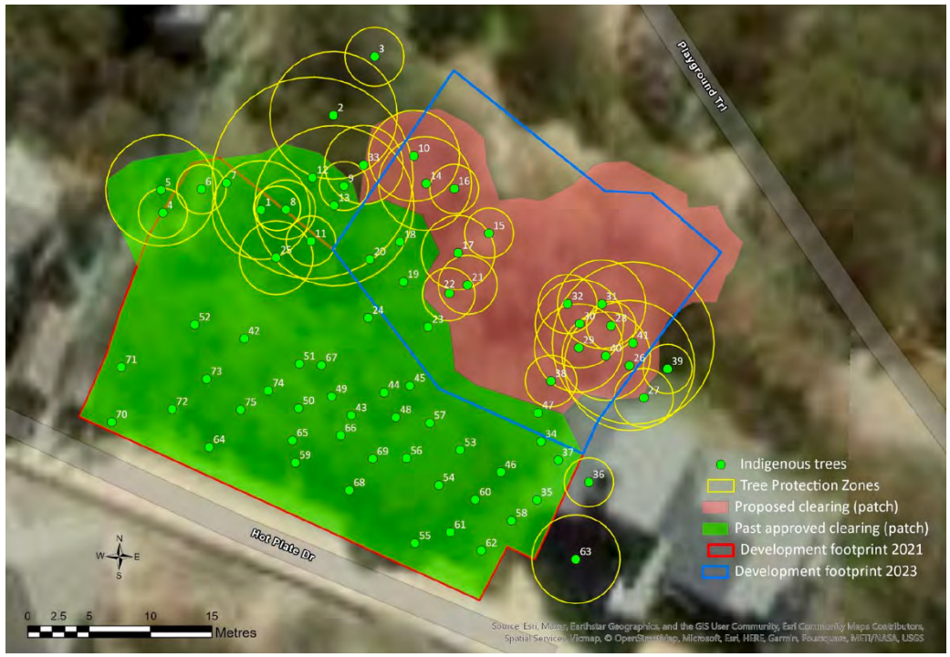
Figure 2: Aerial imagery of the assessed leasehold land on Hot Plate Drive, showing the proposed development footprint and location of assessed trees and pertinent Tree Protection Zones (Image from ESRI Australia 2023).
