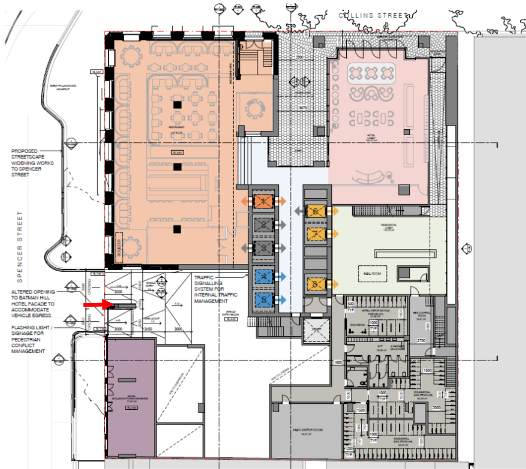
Figure 42 Blade wall retained with new façade opening indicated by the red arrow Source: Carr Architects
