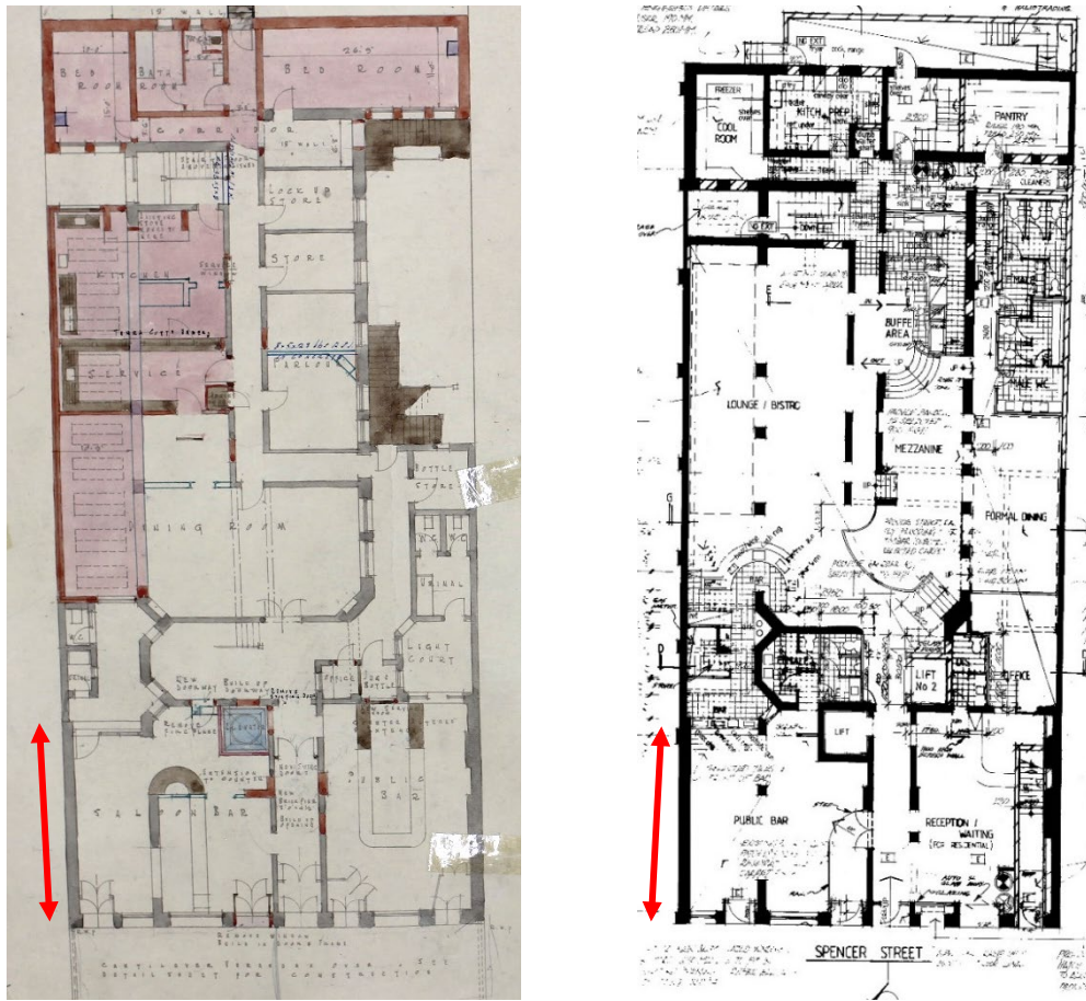
Figure 35 Comparison between 1926 and 1987 ground floor plans, showing the depth of structure to approximately 8.5 metres
