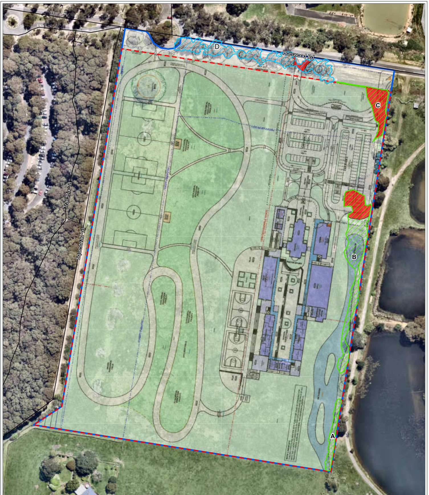
Figure 2: Native vegetation to be removed
