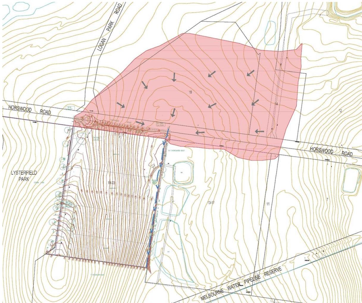
**Figure 3: External Drainage Catchment Plan**
