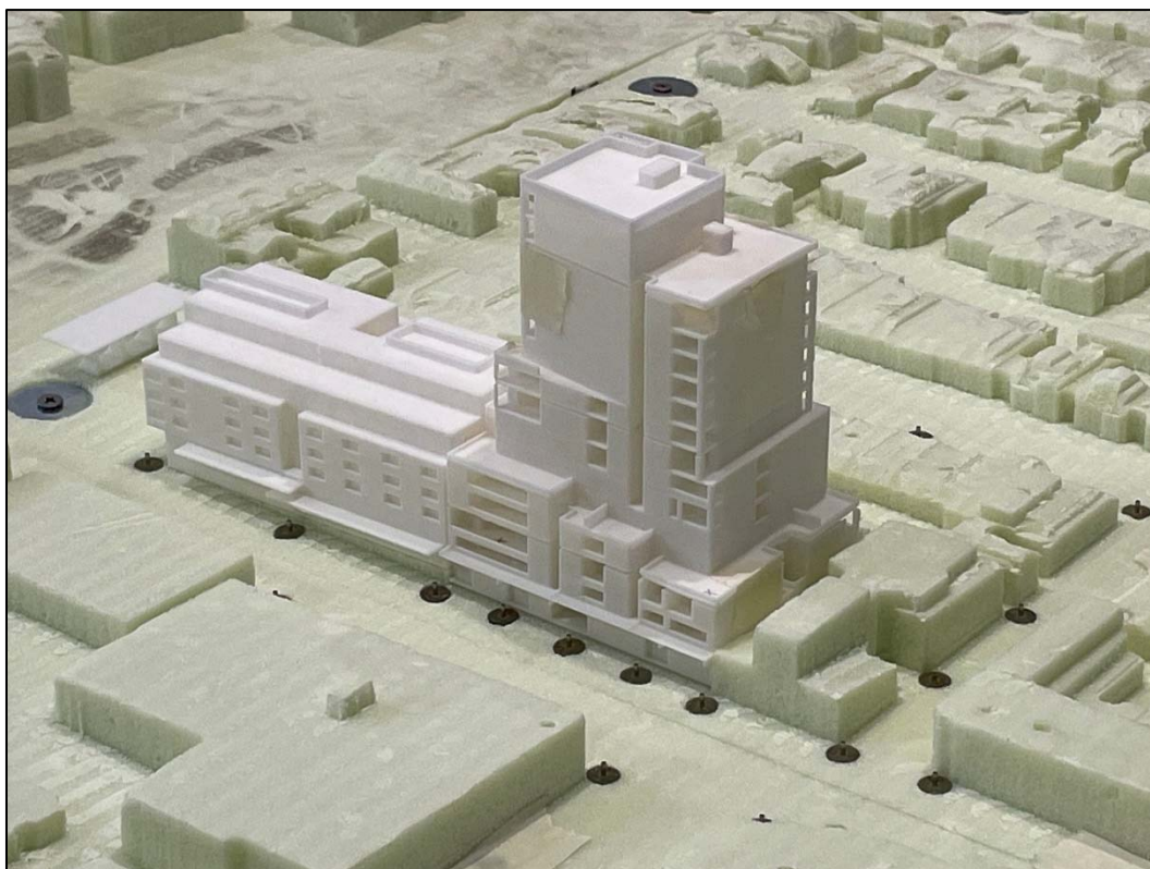
Figure 2c - Close-up view from the southwest of the 1/400 scale model of the proposed 846-858 Glenferrie Road development in the wind tunnel.
