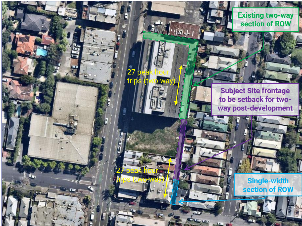
Figure 17: Expected Traffic Volumes in ROW (source: Nearmap.com)
