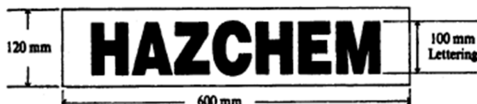
Figure 5-4 Form and dimensions of outer warning placard
