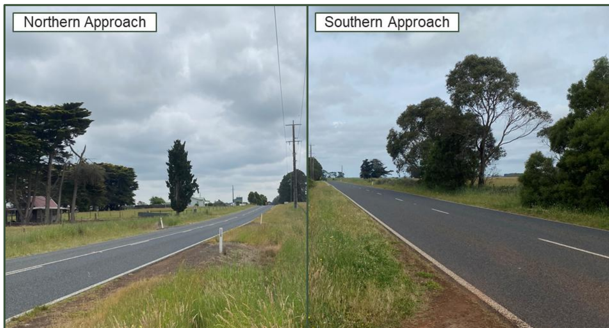
Figure 12 Sight Distance at Proposed Site Access
