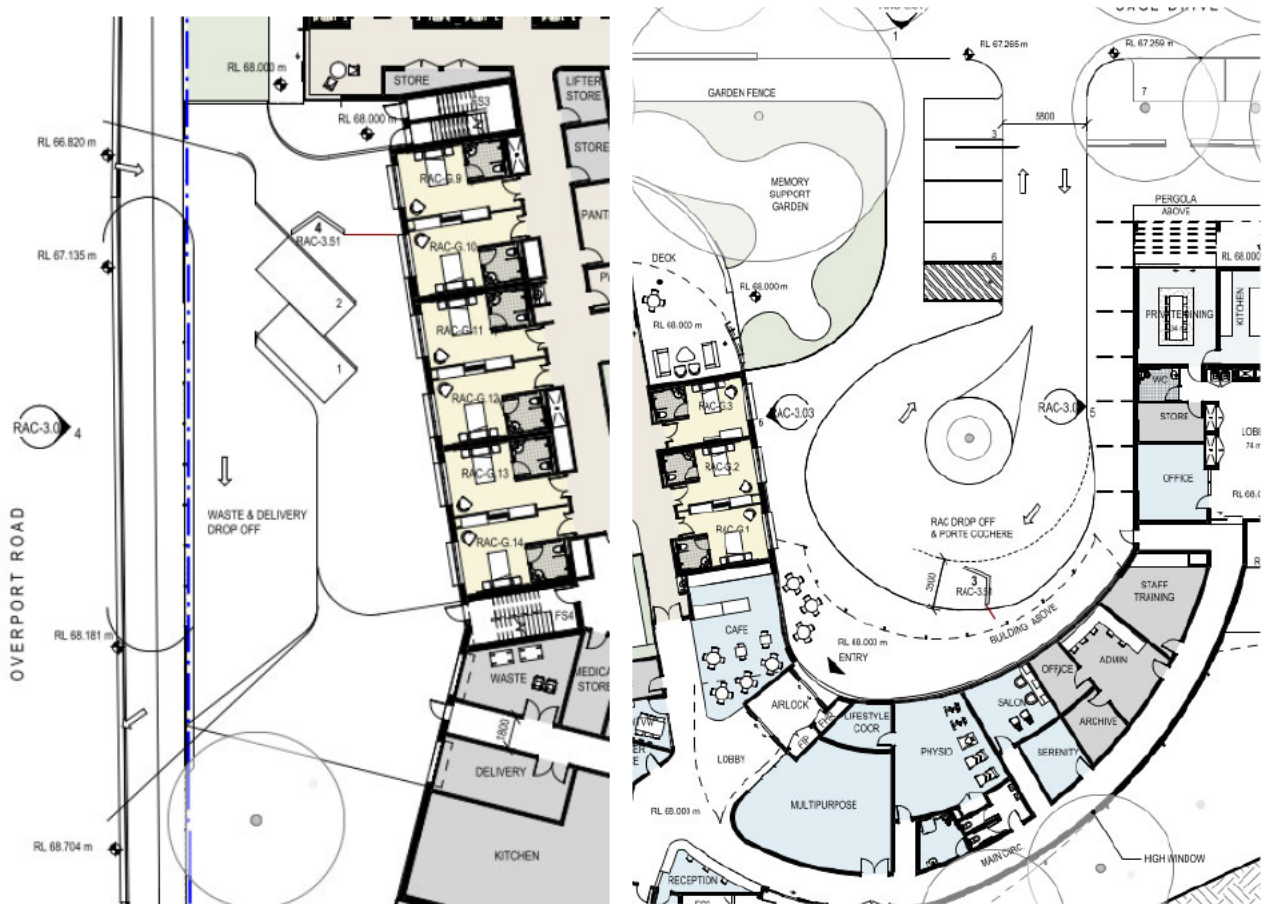
Figure 40 – Excerpt from RAC and ALA building development plans showing proposed new crossovers to Overport Road (left) and proposed RAC/ALA porte cochere for resident on-site pick-up/drop-off and emergency access.
