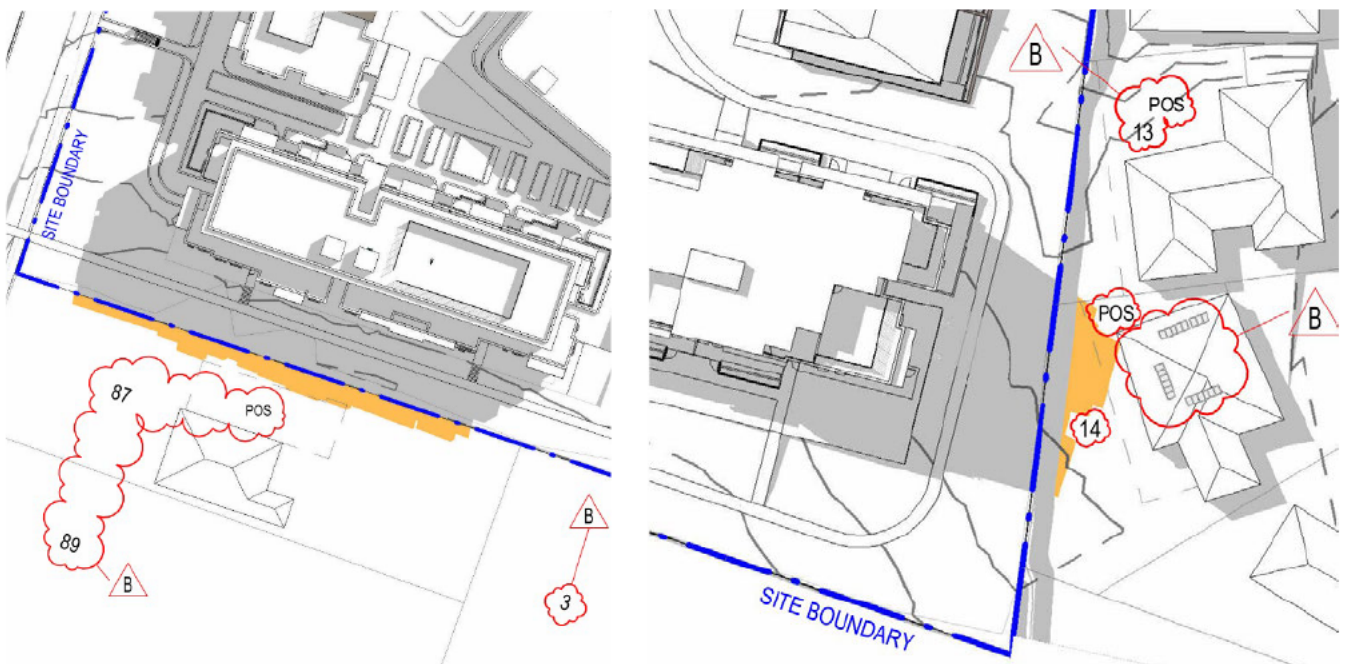
Figure 39 – Excerpt from overshadowing diagrams showing the extent of shadows cast on adjoining properties at 9am (left) and 3pm (right) (Source: Masterplan prepared by Thomson Adsett)
