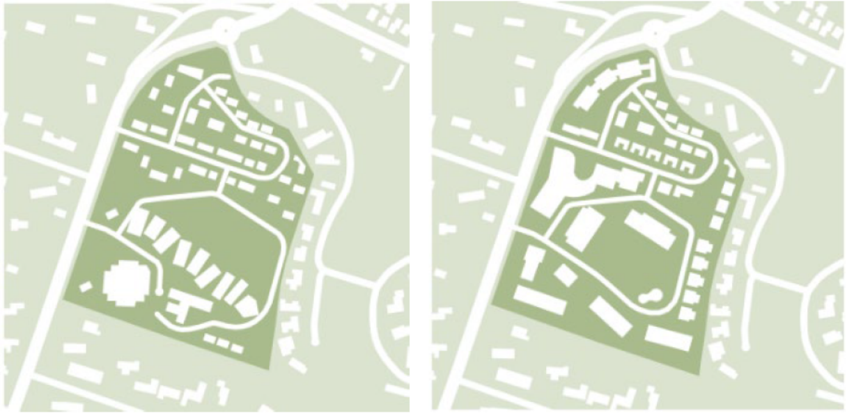
Figure 23 – Comparison of permeable and/or green space across the existing site (left) and proposed development (right) (Source: Architectural Report, prepared by Thomson Adsett)
