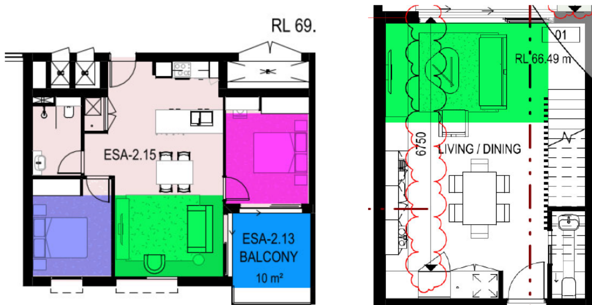
Figure 38 – Excerpt from ESA Apartment development plan demonstrating compliant living and bedroom areas required by Clause 58 Function Layout standard (right) and area within ESA Townhouses living which meets minimum area and dimension for Function Layout standard (left)
