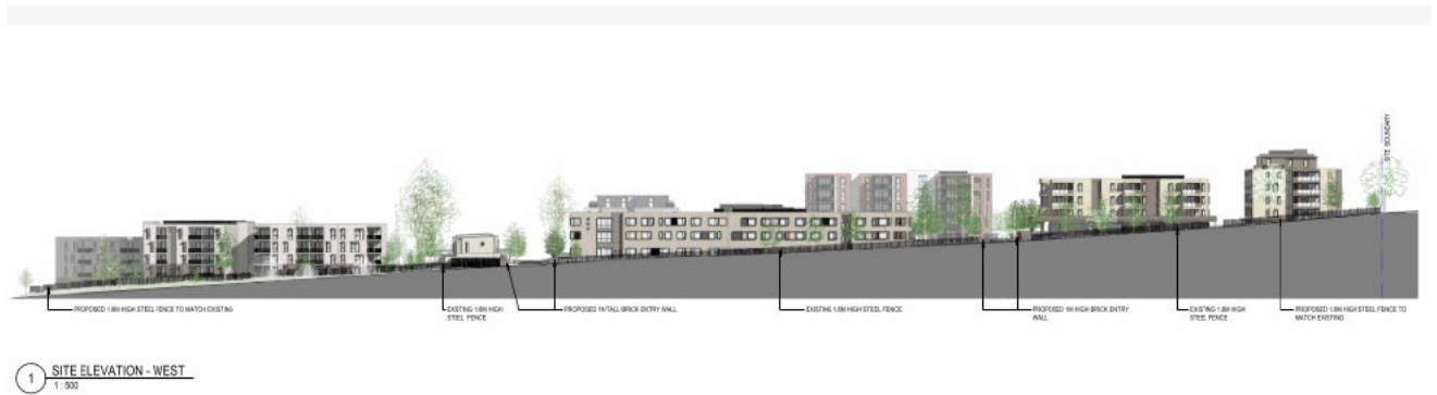
Figure 27 – Overall Overport Road elevation showing the transition in height with the fall of the land(right to left) of Buildings C3, C1, RAC, Block E and ESA Apartments (Source: Architectural Report, prepared by Thomson Adsett)
