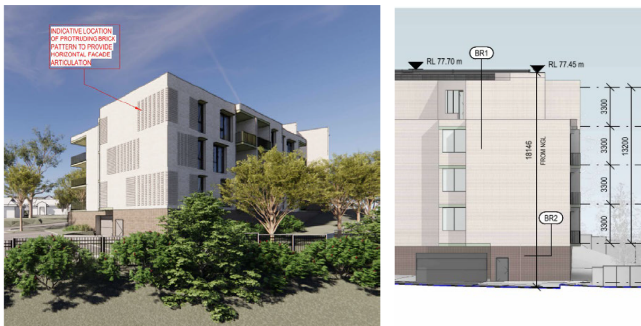
Figure 30 – Excerpt from discussion plan demonstrating proposed façade articulation to ESA Apartments which is to be secured via conditions (left) and excerpt from ESA Apartments plan demonstrating the existing presentation of the sheer 4-storey wall.
