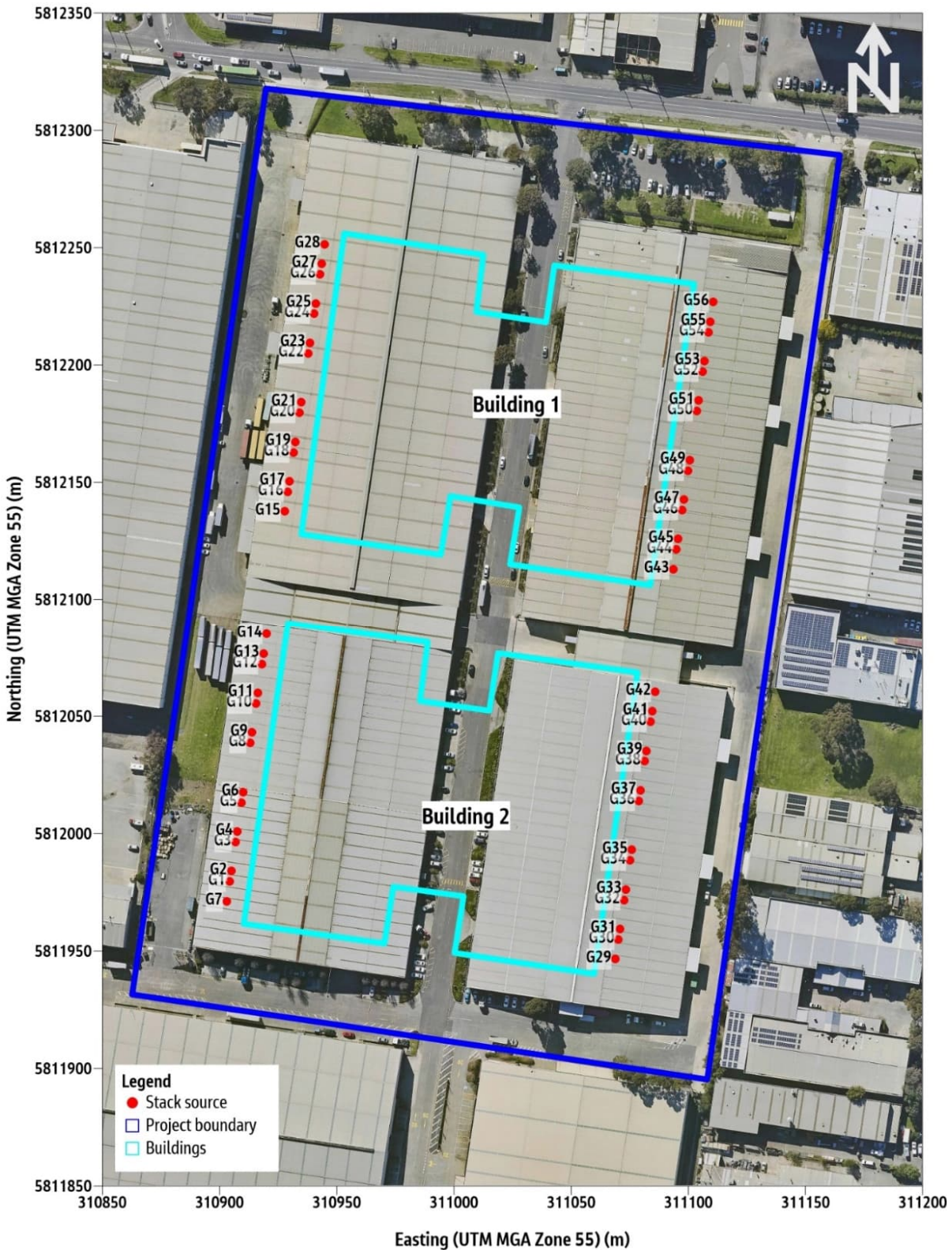
Figure 4-1. Source arrangement, proposed Brooklyn data centre
