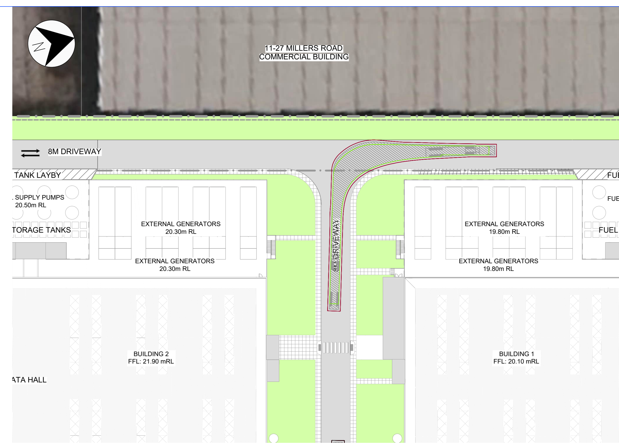
SWEPT PATH TRACKING 2: 19m PMS SEMI TRAILER - RIGHT TURN NORTH TO FRANCIS ST EXIT SCALE: 1:500
