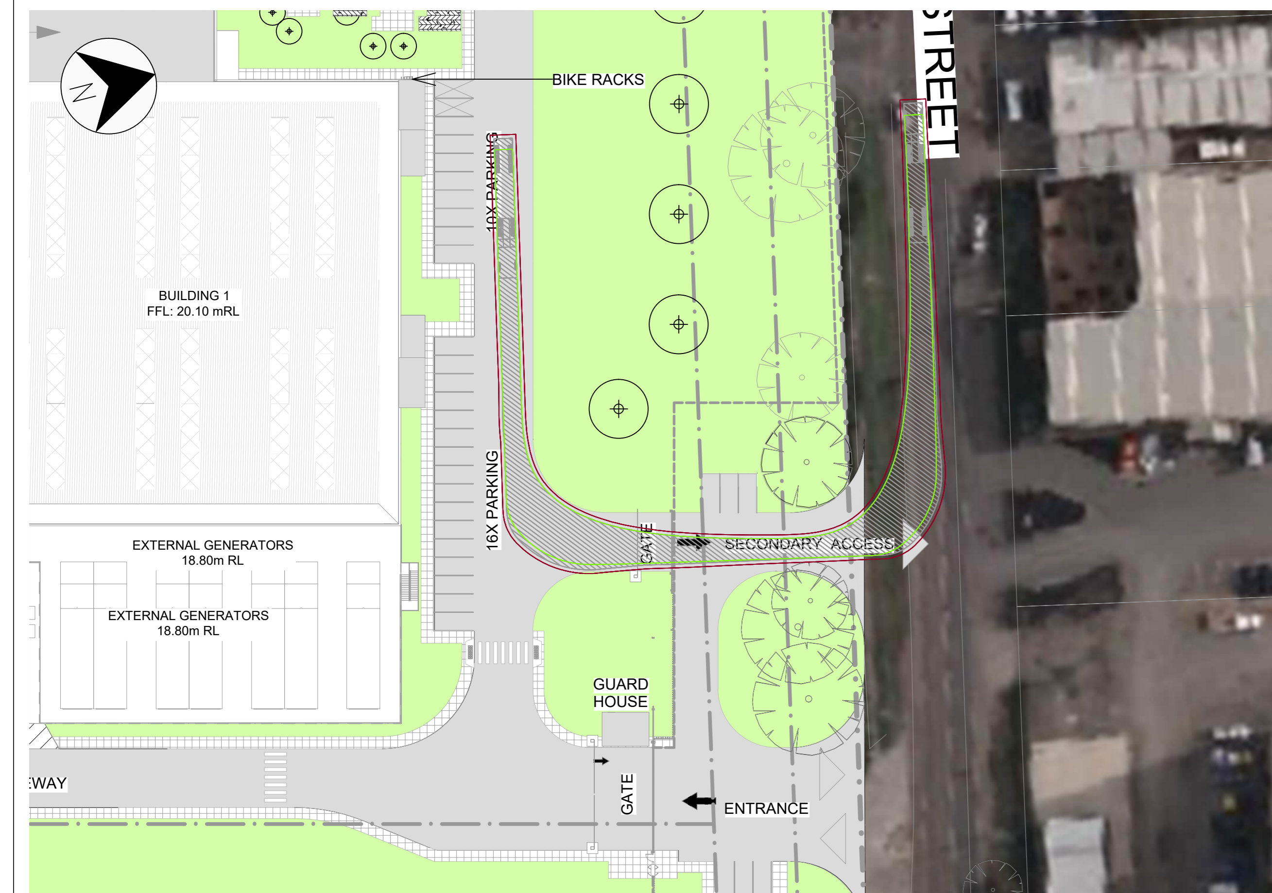
SWEPT PATH TRACKING 3 19m PMS SEMI TRAILER - EXITING ONTO FRANCIS ST VIA SECONDARY EXIT SCALE: 1:500
