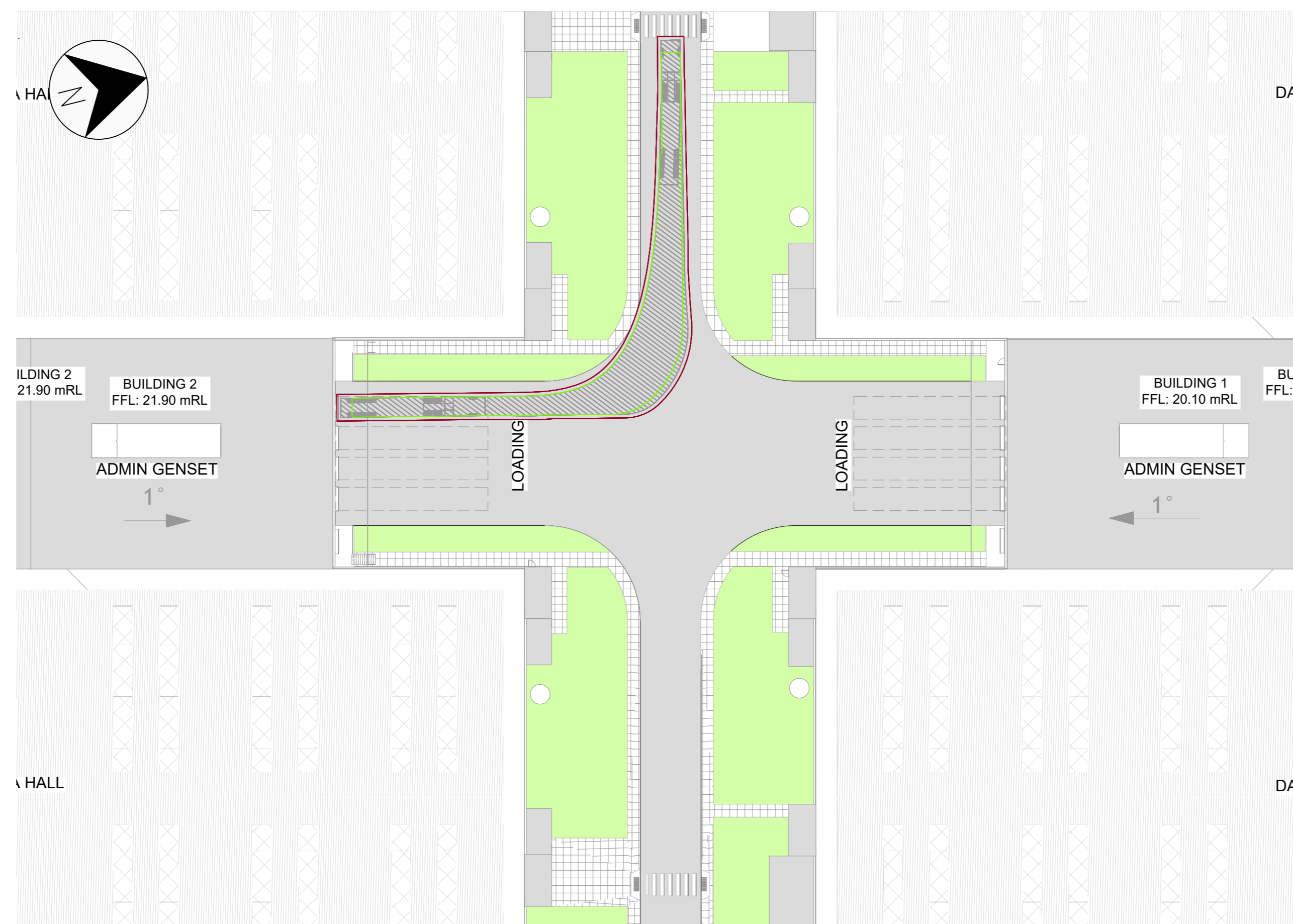
SWEPT PATH TRACKING 6: 19m PMS SEMI TRAILER - EXITING LOADING BAY 2-4 SCALE: 1:500
