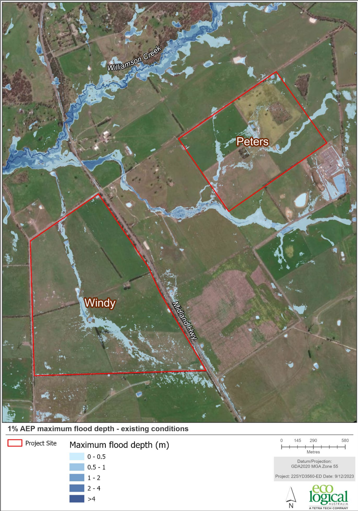
Figure 5-4 1% AEP maximum flood depth – existing conditions
