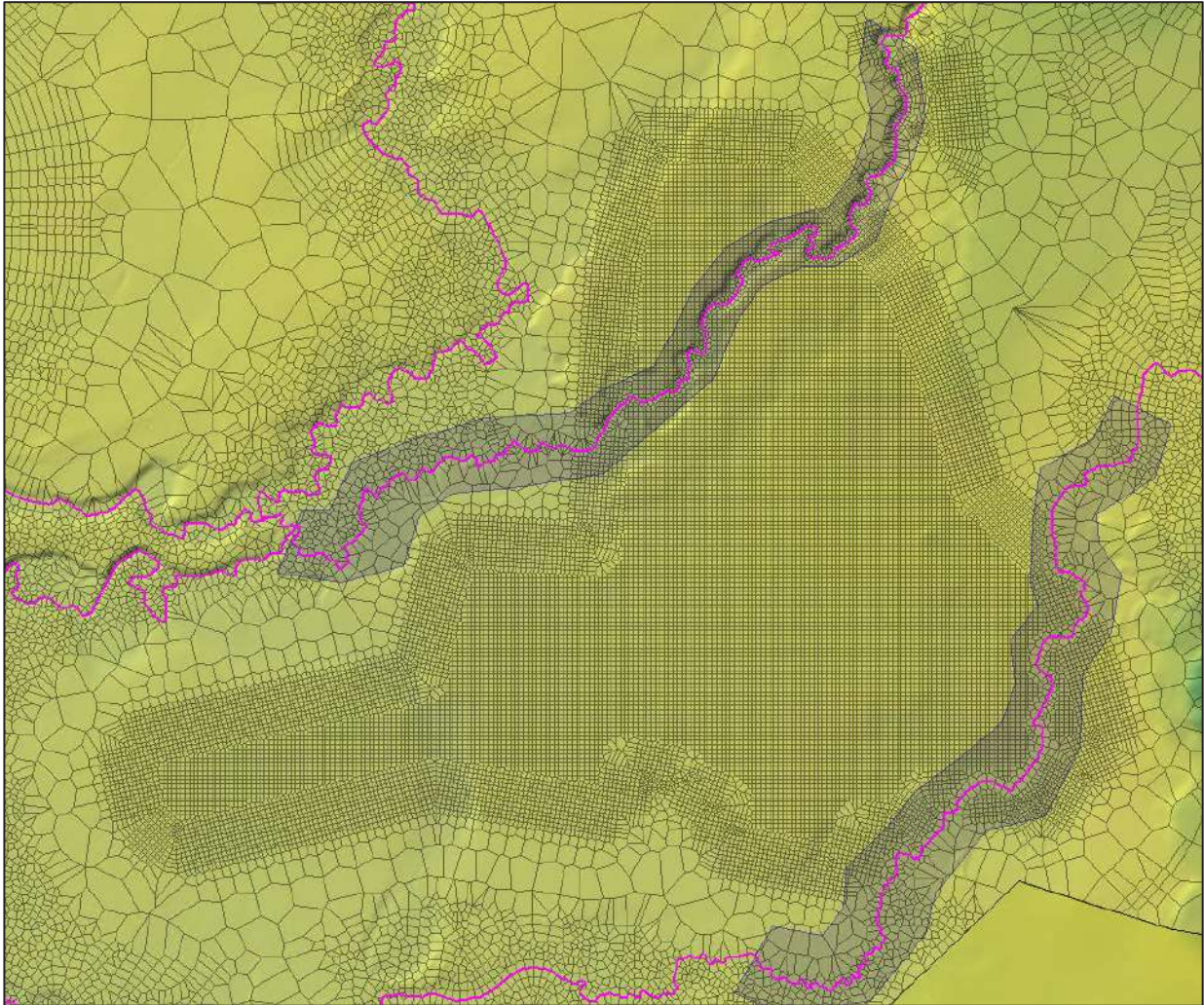
Figure 4-4 Manning's n roughness coefficient specification (green is 0.08, blue is 0.06)
