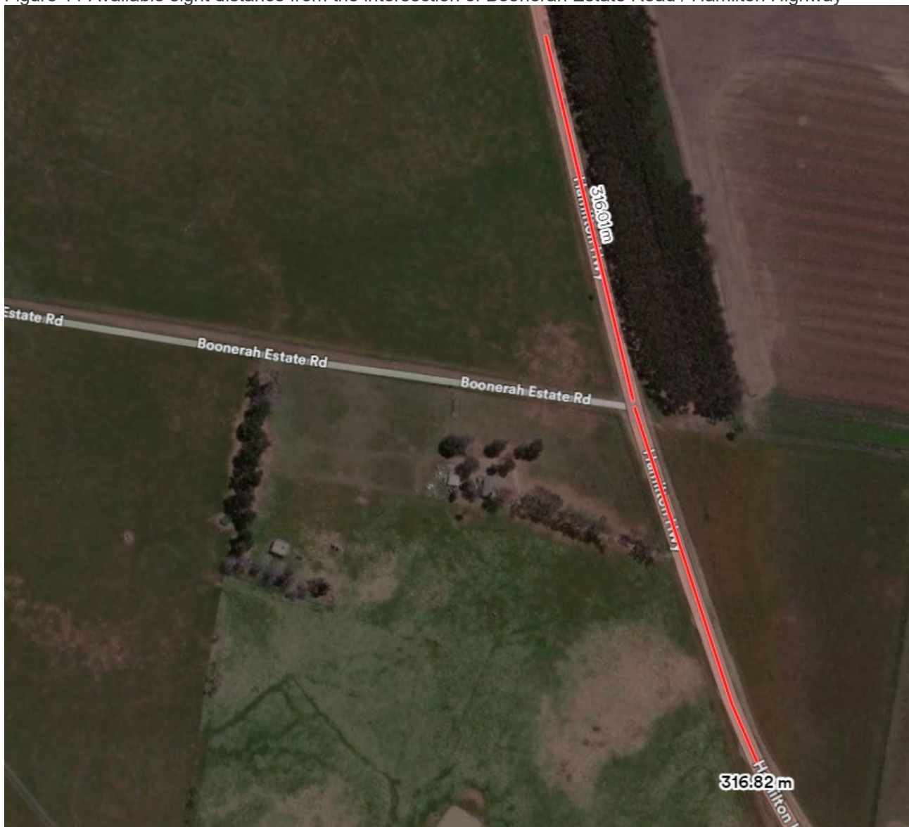
Figure 11 Available sight distance from the intersection of Boonerah Estate Road / Hamilton Highway
