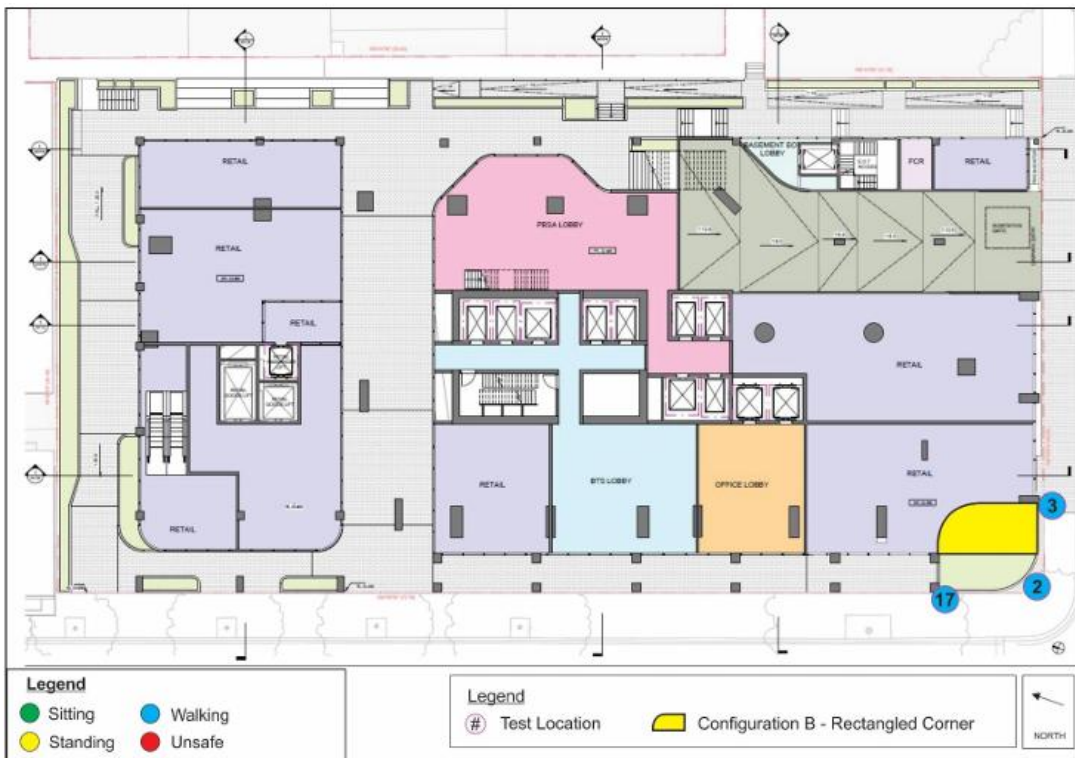
Figure 31: Proposed south-west corner wind comfort criteria satisfied (Source: Application - Environmental Wind Conditions Study)
