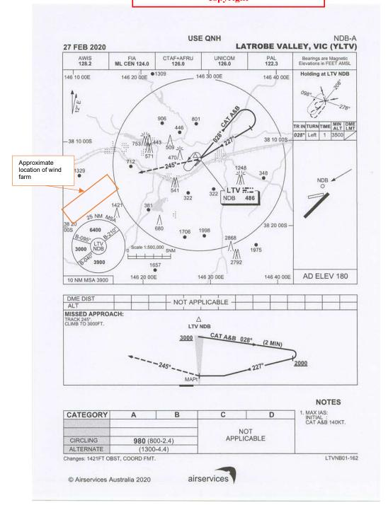
Figure 7 – YLTV NDB-A Plate with approximate Wind Farm Location8
