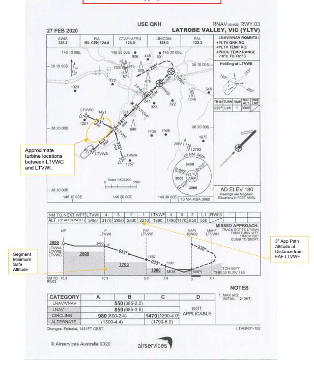
Figure 5 – YLTV RNAV RWY03 Instrument Approach Plate7
