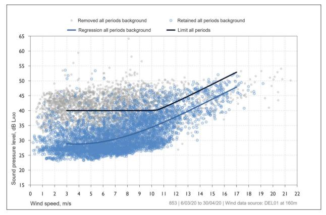
Figure 21: Receiver 853 night-time periods – derived background noise levels and noise limits
