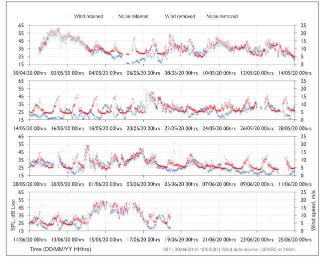
Note: Based on observations while in attendance at the site and our review of sample audio recordings, the minimum measured noise levels of the order of 25 dB L<sub>A90</sub> are most likely to relate to domestic equipment (A/C unit) at the property. The noise contribution of this equipment does not sufficiently influence the derived background noise levels and noise limits presented in the figures below.
