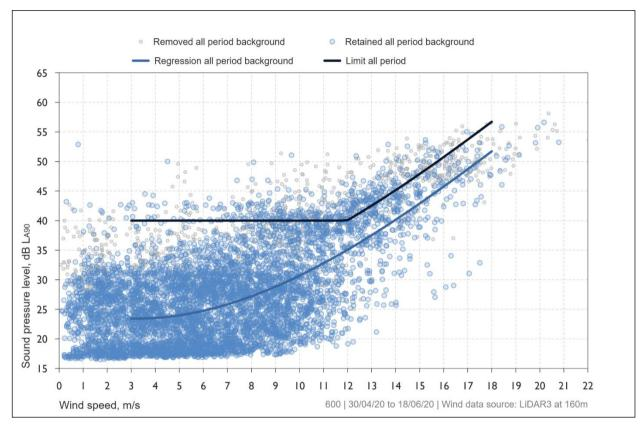
Figure 5: Receiver 600 night-time periods - derived background noise levels and noise limits
