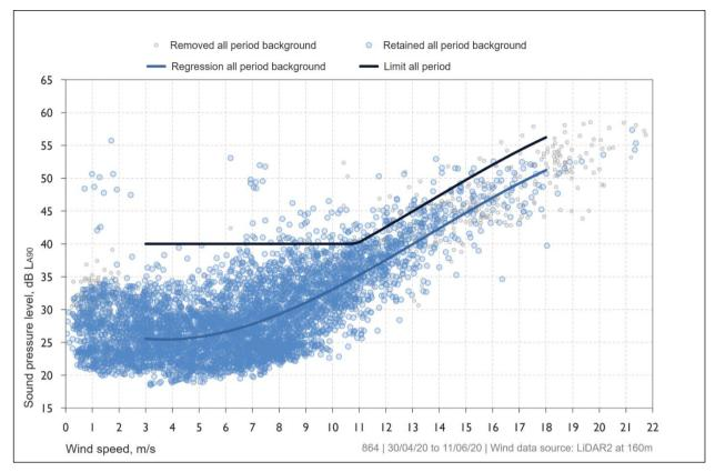
Figure 25: Receiver 864 night-time periods - derived background noise levels and noise limits
