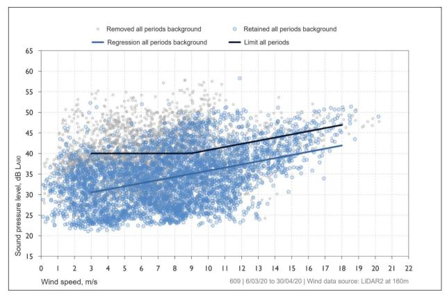
Figure 9: Receiver 609 night-time periods - derived background noise levels and noise limits
