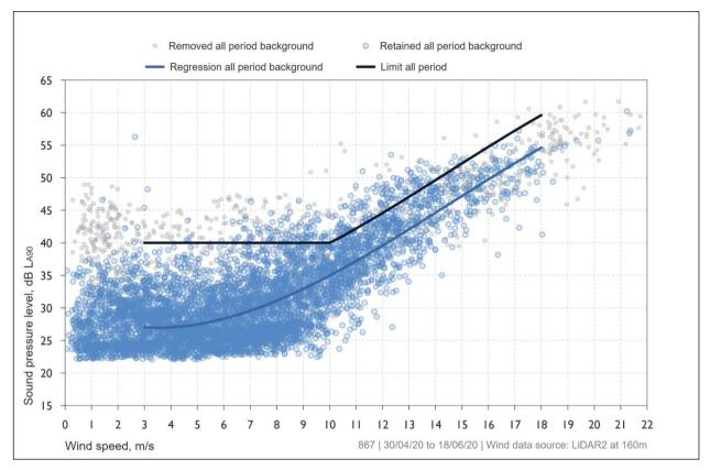
Figure 29: Receiver 867 night-time periods – derived background noise levels and noise limits
