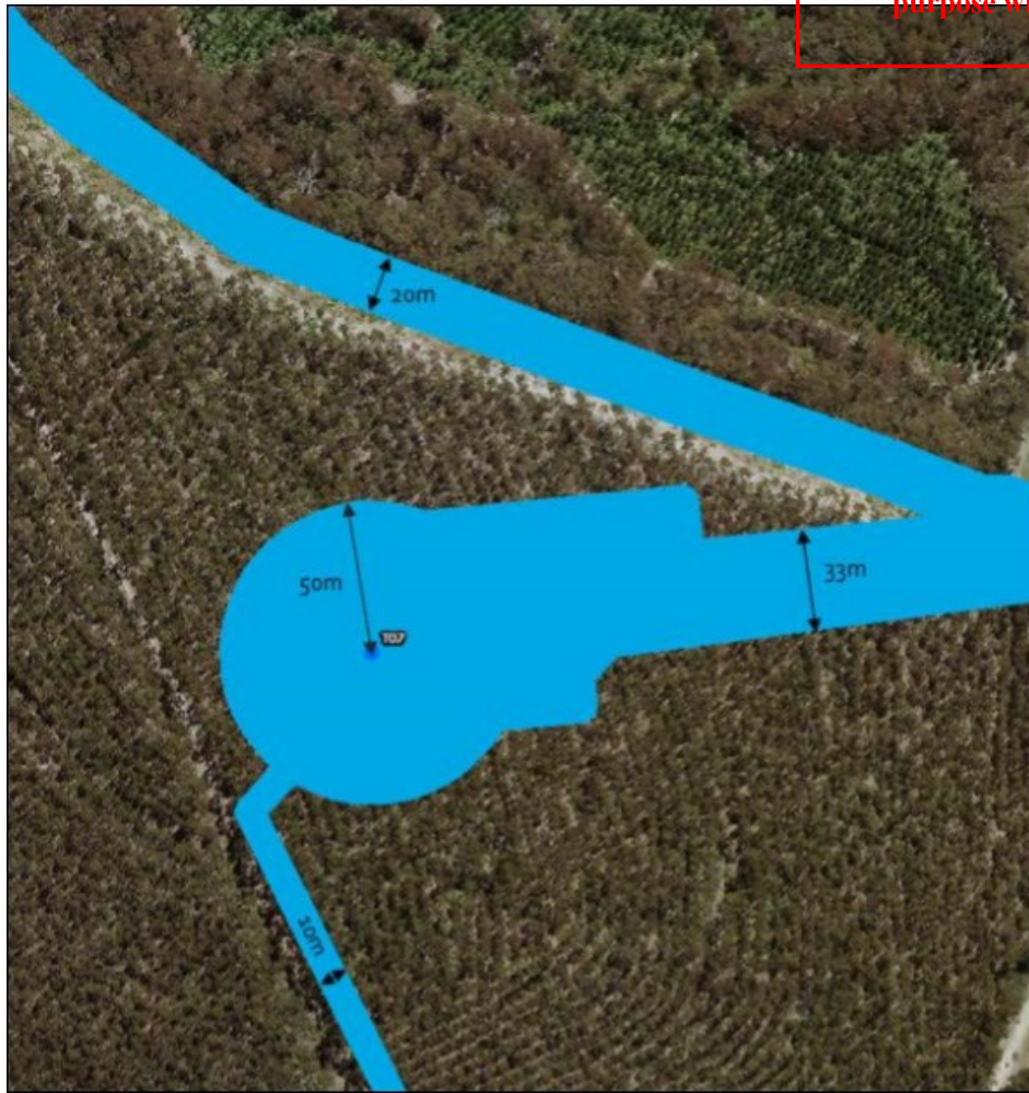
Figure 16 - Example of plantation fuel modification for proposed tower
