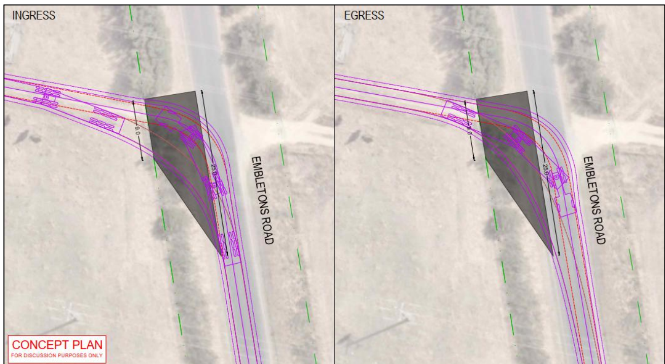
Figure 5-5 26.0m B-Double Construction Site Access Ingress/Egress – Eastern Side
