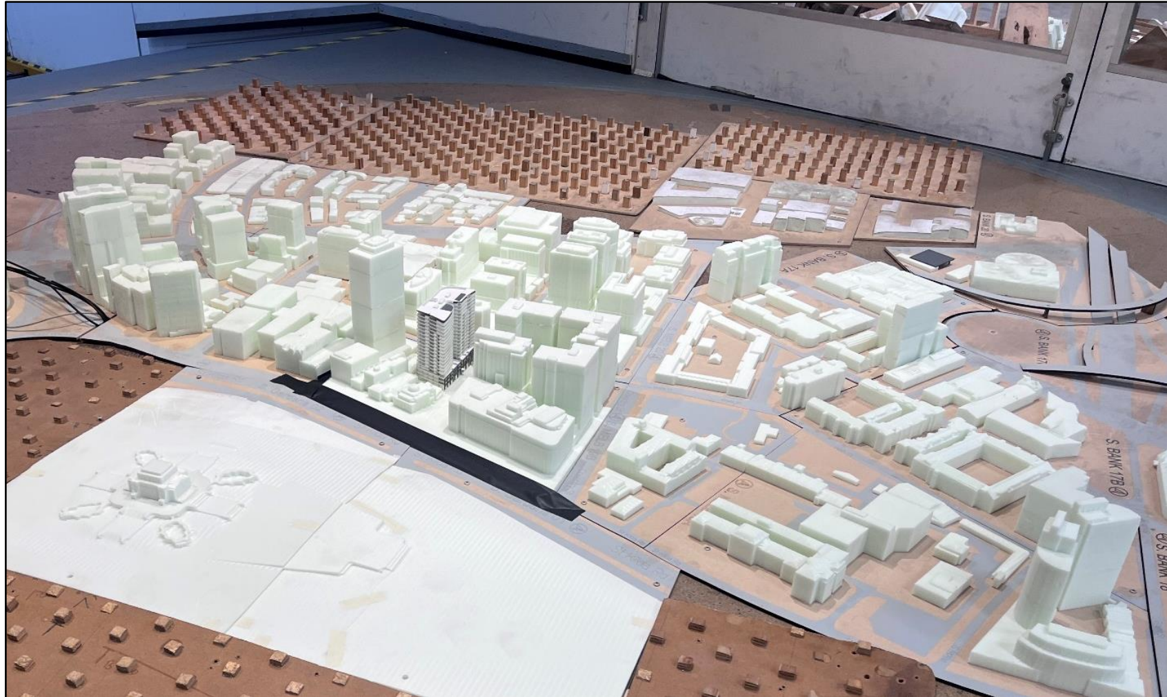
Figure 3 - View from the northeast of the 1/400 scale model of the proposed 11-27 Dorcas Street Development in the wind tunnel.
