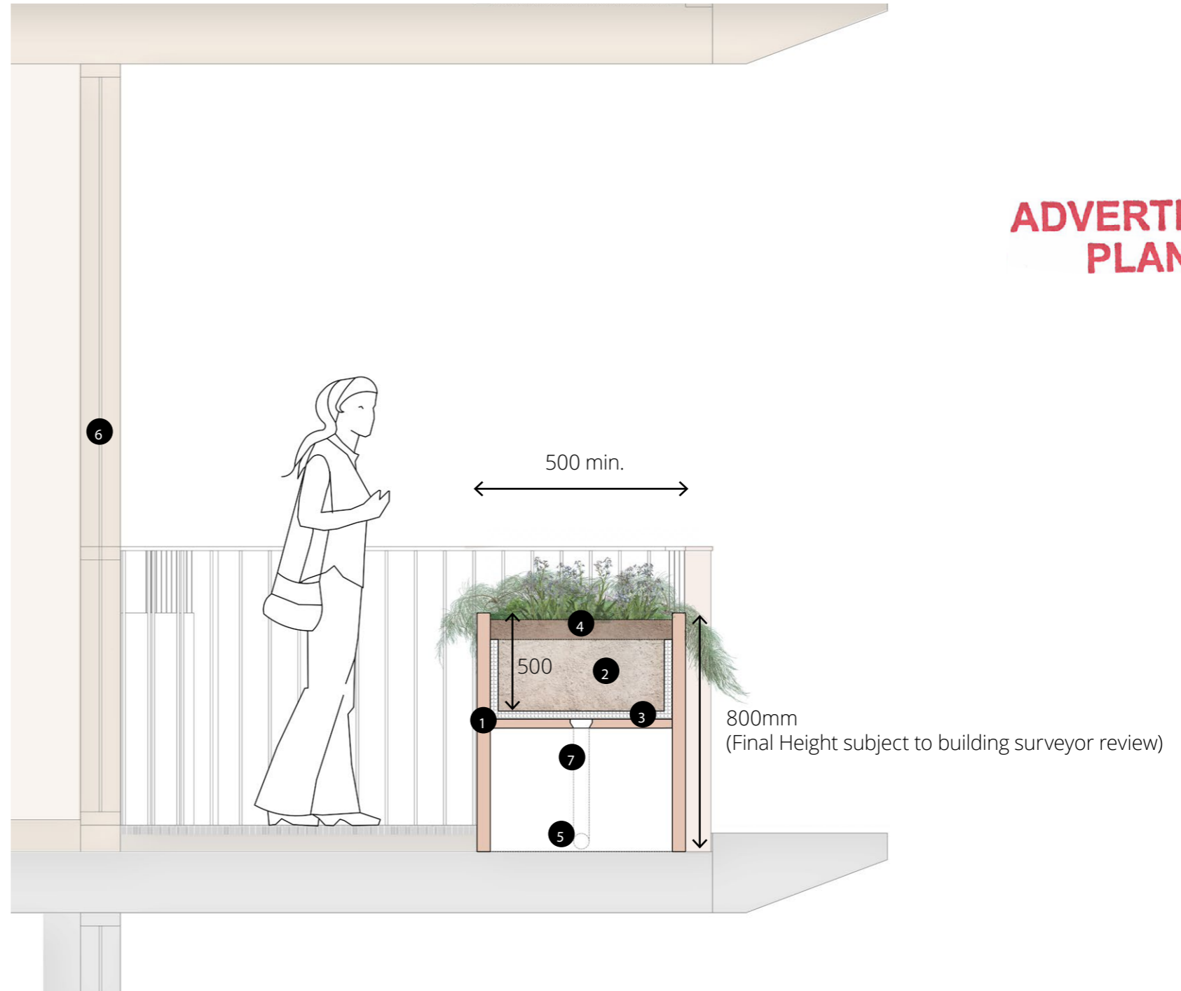
Terrace Edge Planter Typical Section
