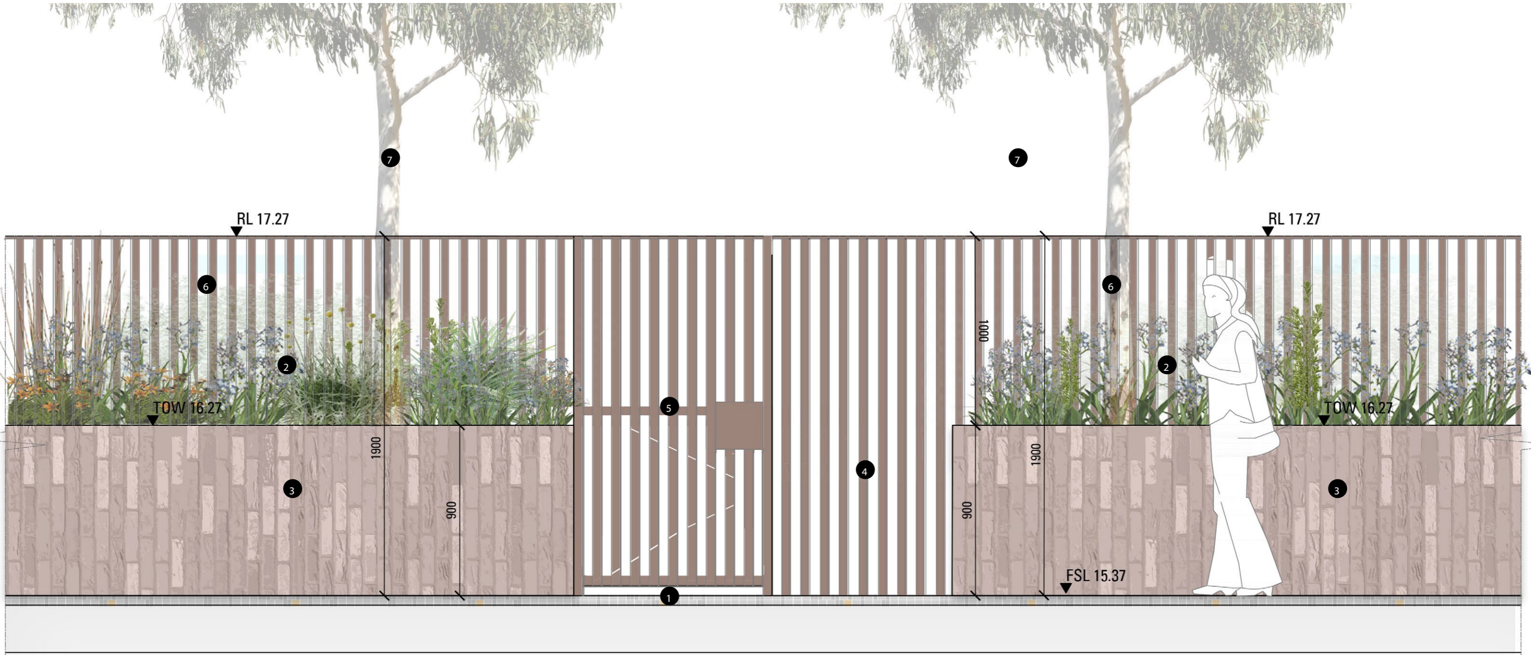
Steel Palisade Fence (0.8m) on top of Planted Raised Garden Bed Wall (1.0m) | Entry Gate & Fence | Steel Palisade Fence (0.8m) on top of Planted Raised Garden Bed Wall (1.0m)
