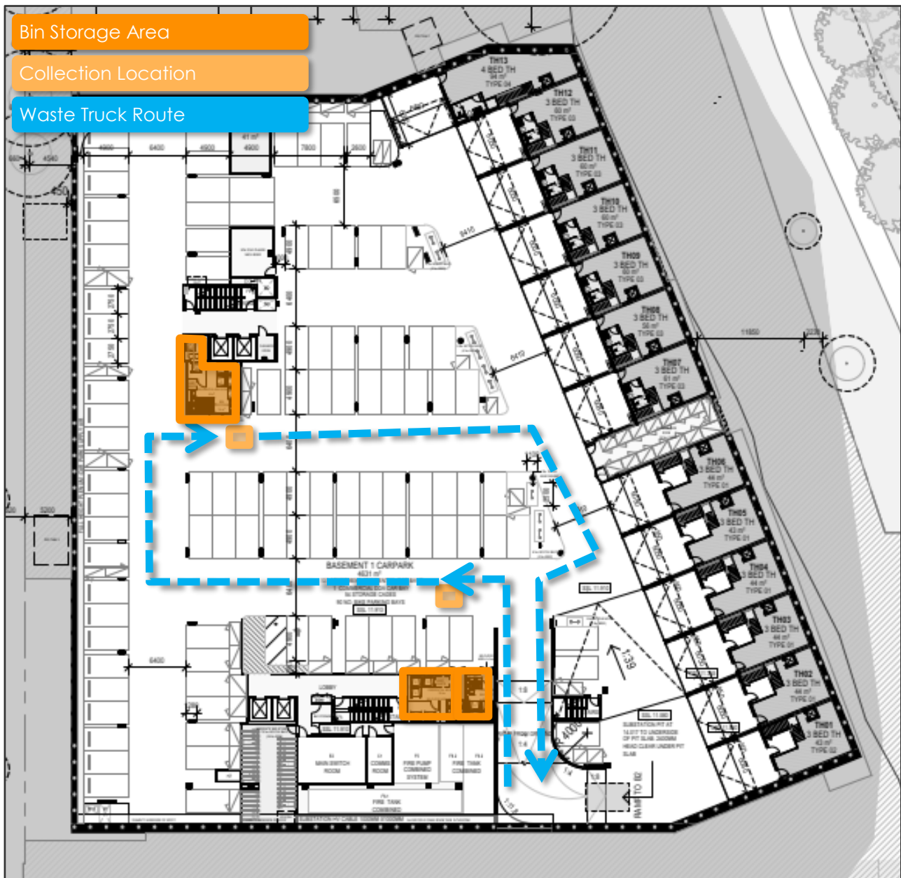
Figure 3 Bin Storage Room and Collection Details
