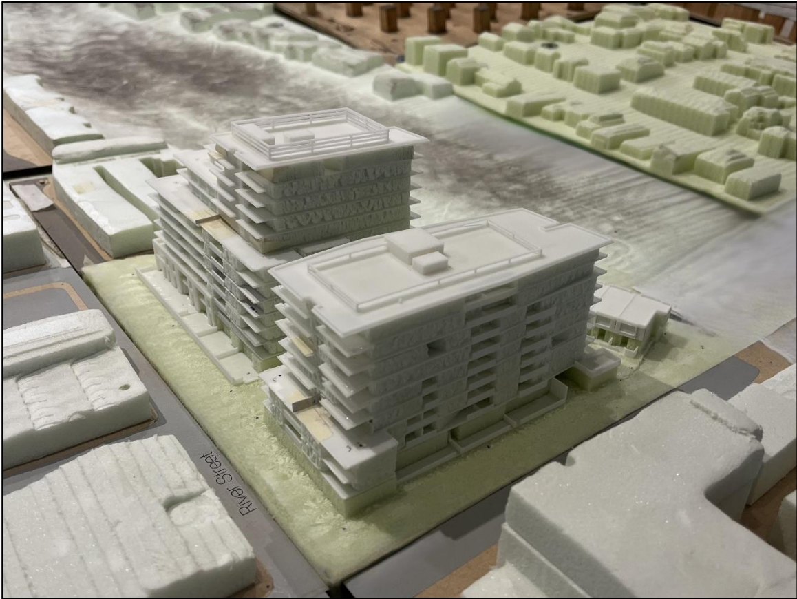
Figure 2d - Close-up view from the southwest of the 1/400 scale model of the proposed 43 and 63-67 River Street development in the wind tunnel.
