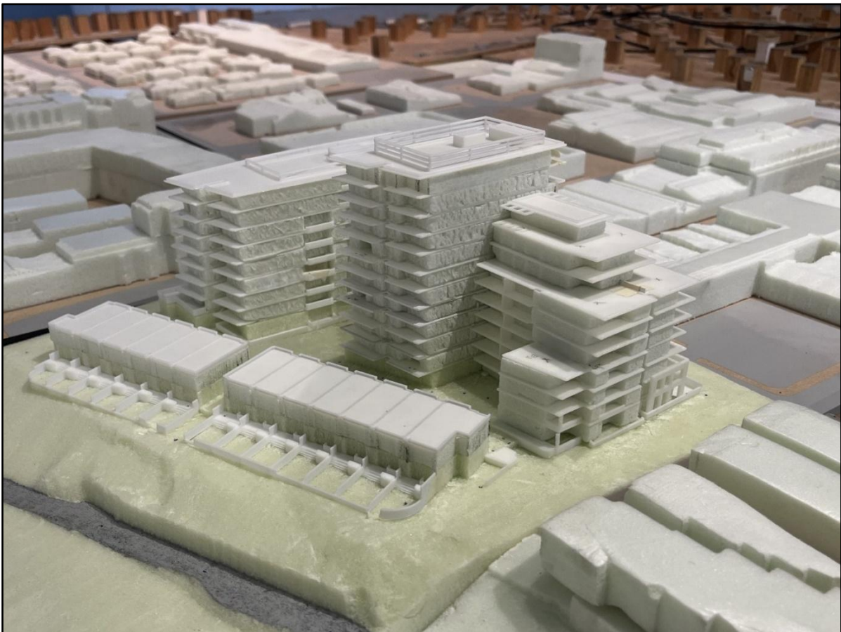
Figure 2a - Close-up view from the northeast of the 1/400 scale model of the proposed 43 and 63-67 River Street development in the wind tunnel.
