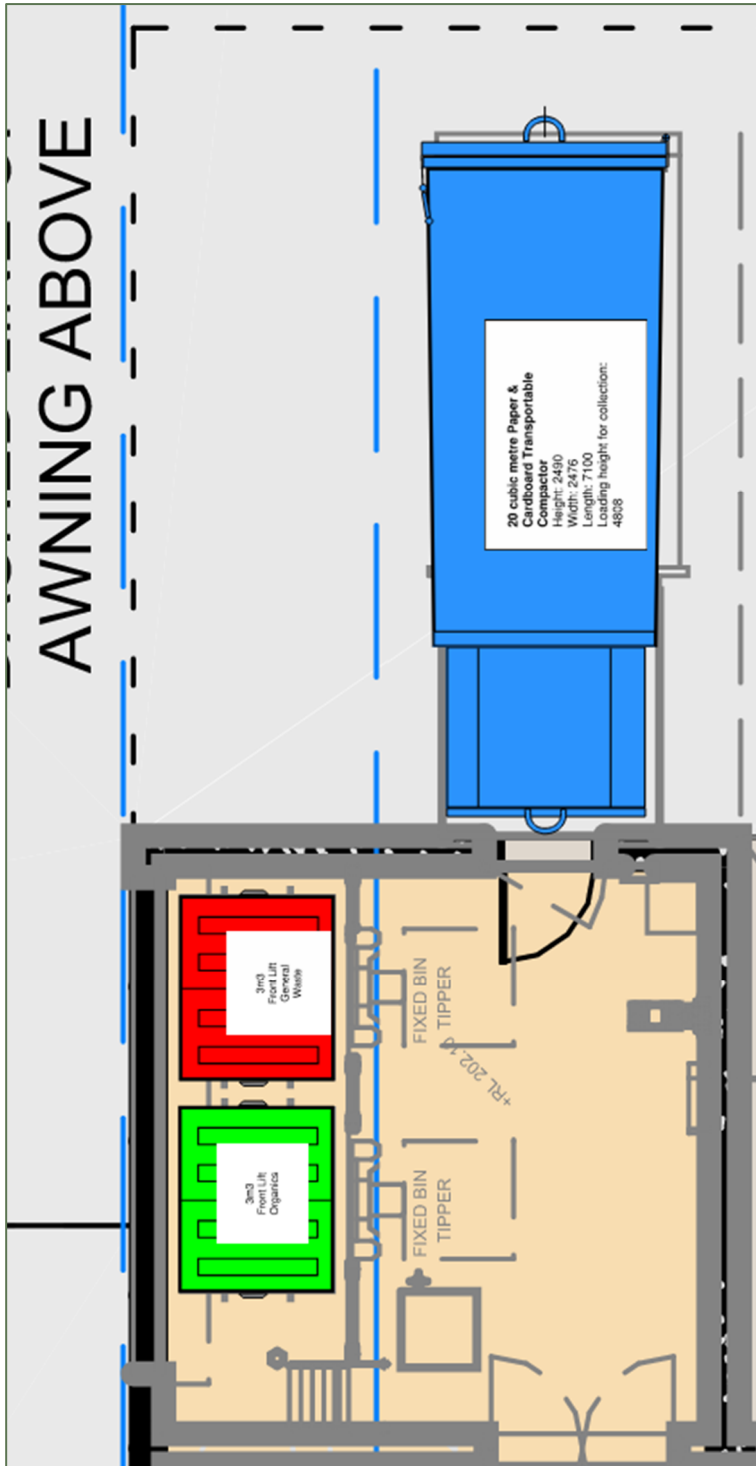
Figure 4.1: Woolworths Supermarket - Waste Equipment Location and Layout
