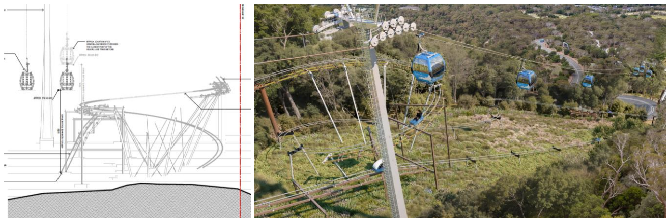
Above: Section drawing of proposed luge below gondolas (left) and 3D render of proposed luge corridor (right).
