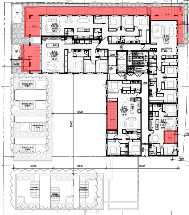
Figure 12: Level 4 floor plan with recommended wind criteria overlaid.
