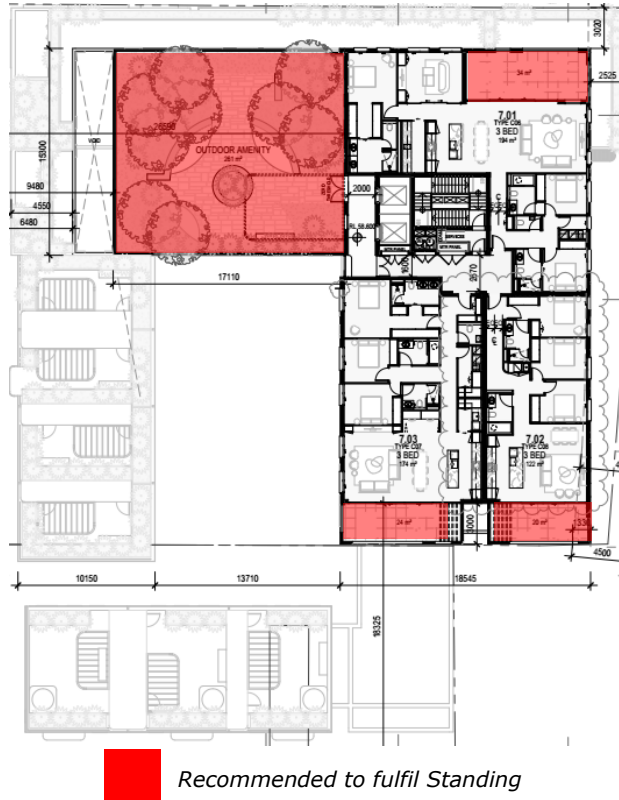
Figure 14: Level 7 floor plan with recommended wind criteria overlaid.
