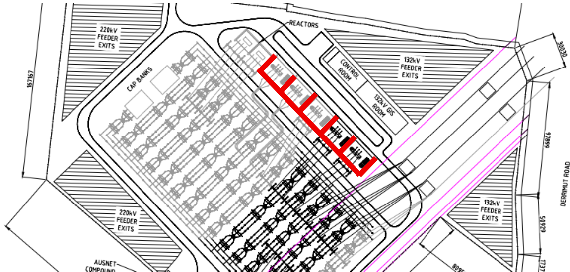
Figure 4: Indicative localised 6.5m acoustic barrier alignment
