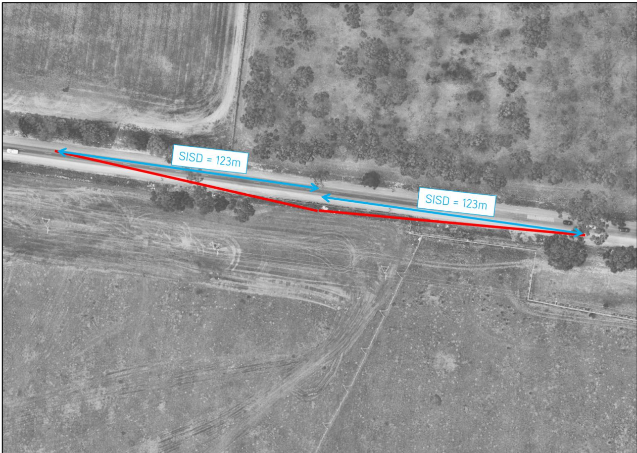
Figure 16 Sight distance diagram
