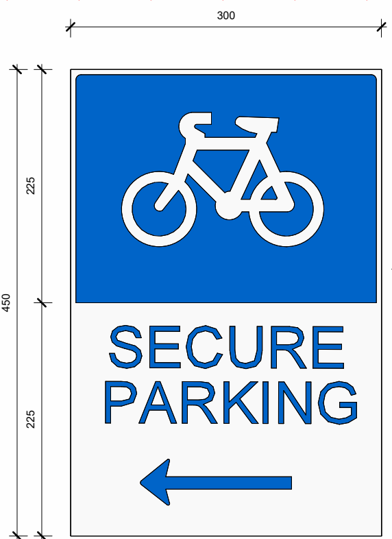
1 Signage Elevation - North - Detail 1 : 10
