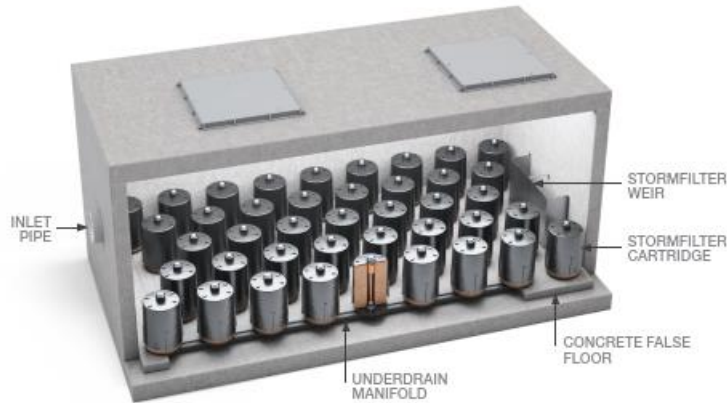
Figure 2: Example conceptual diagram of a StormFilter® system
