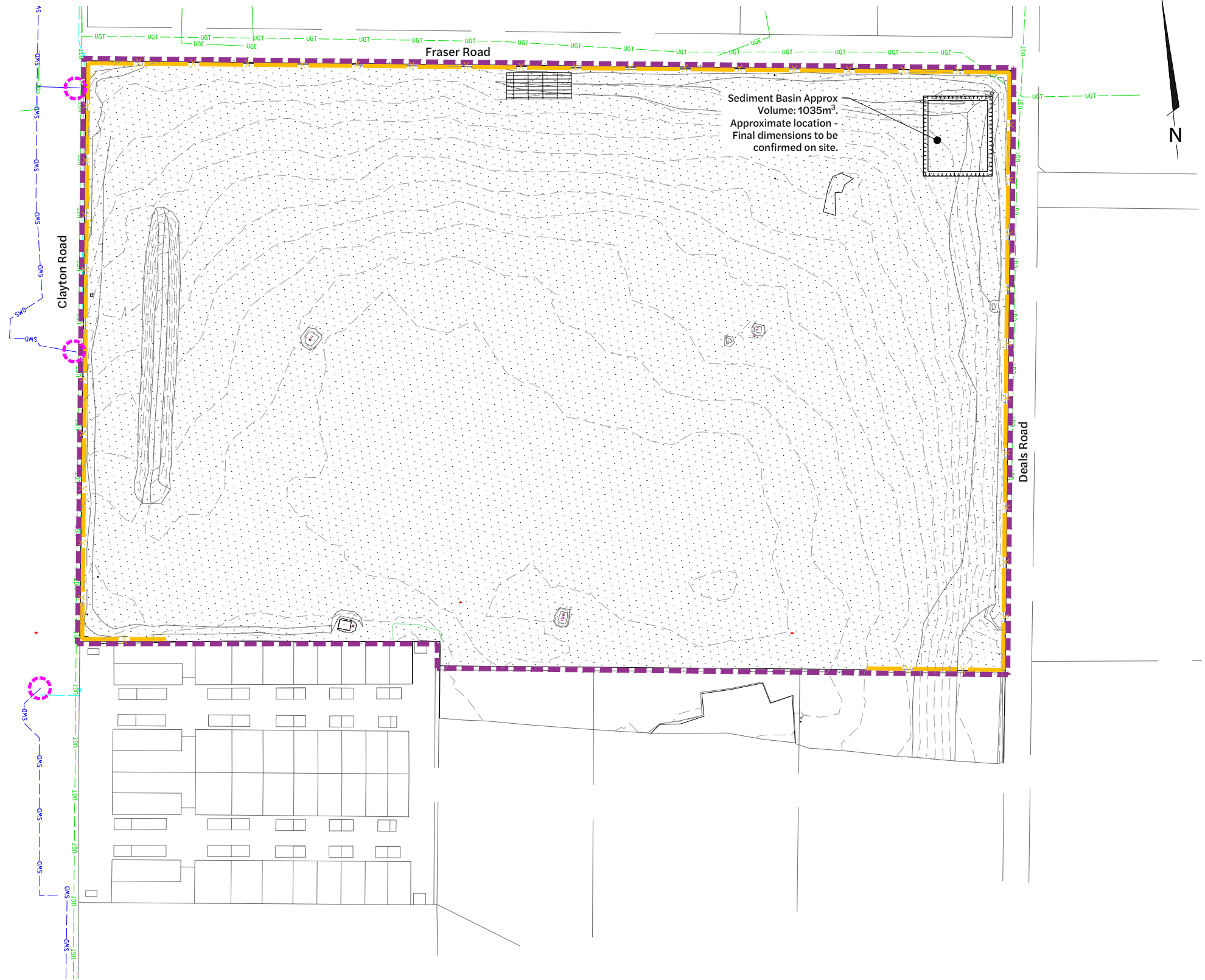
Erosion and Sediment Control Layout Plan 1:1000 Scale
