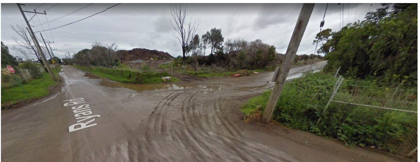
Figure 4-7 Deals Road and Fraser Road Intersection Stormwater Ponding (Source: Google Street View 2009)
