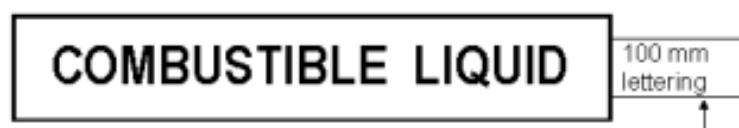
Figure 7 Placard for C1 combustible liquids in bulk
