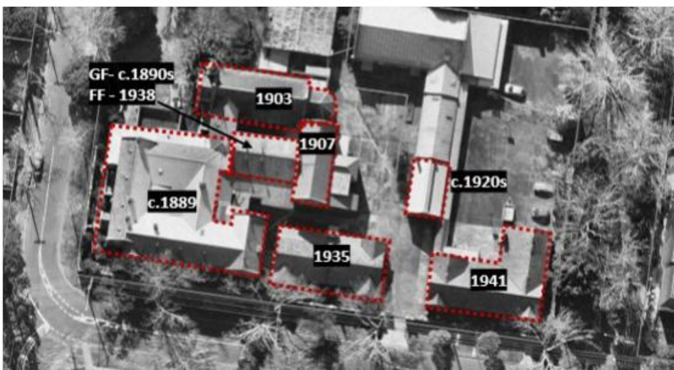
Figure 4. Aerial view of the subject site (part) with dates of construction for the main buildings overlaid (Lovell Chen).
