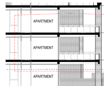
Recessed living areas windows are shaded by the terrace above in.
