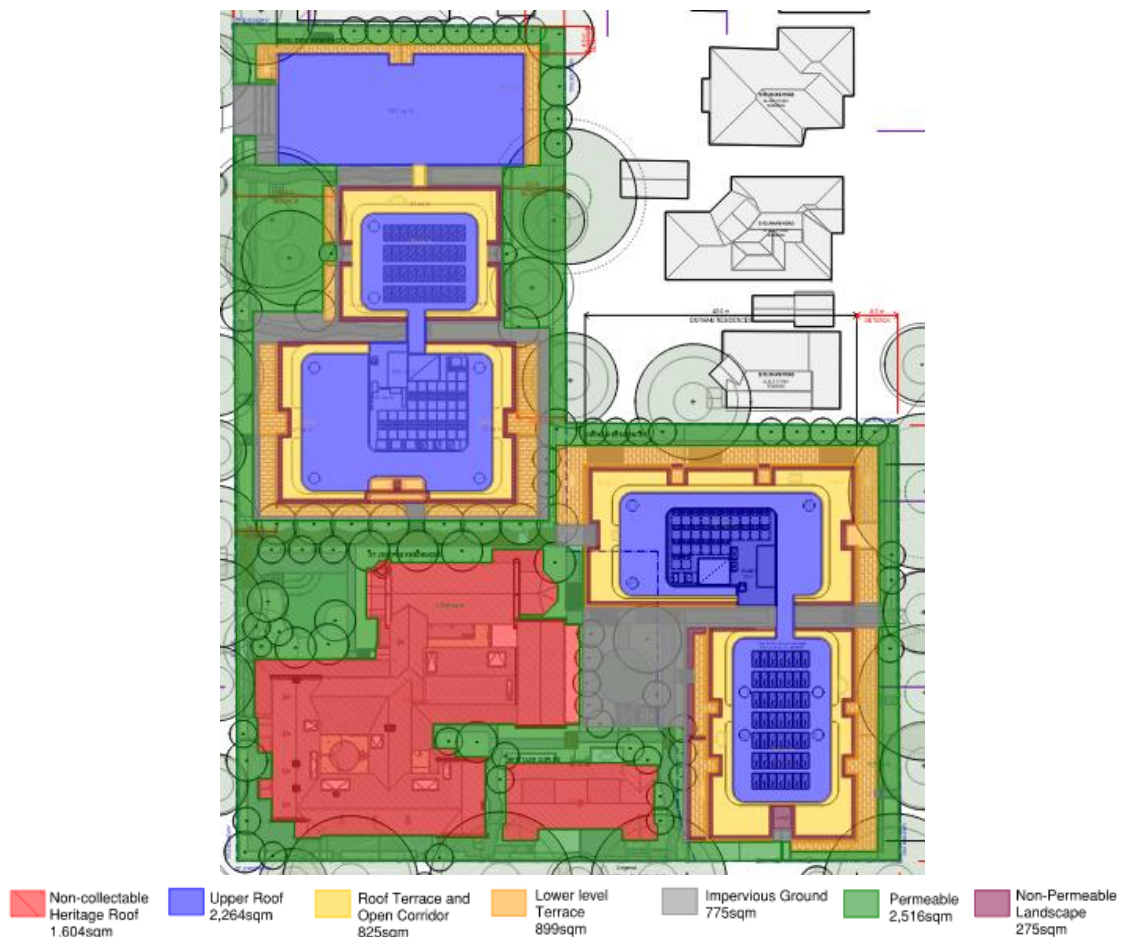
Figure 1 - Mark-up of water catchment and impervious areas
