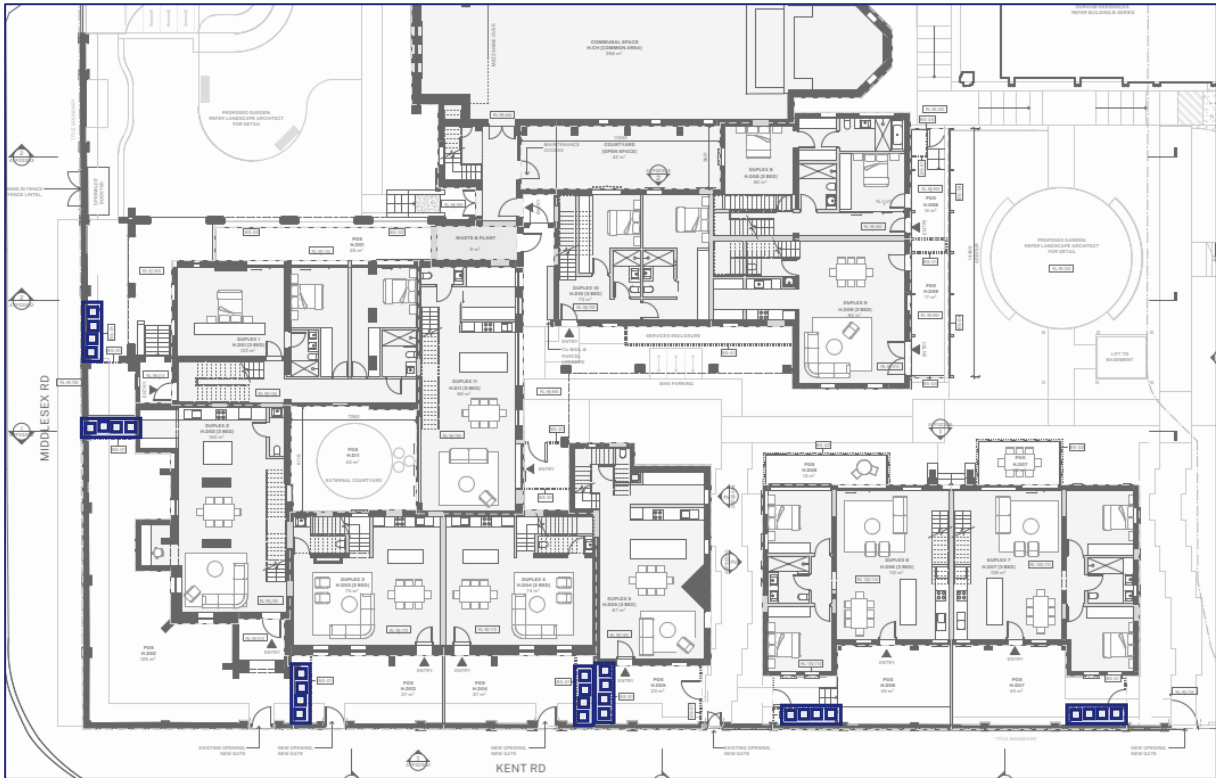
Figure 3: Individual waste enclosures for Building C – (D1-D7)
