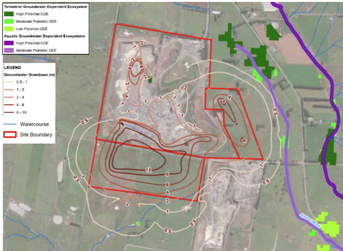
Figure 19 – Excerpt from Groundwater Dependent Ecosystems report show the anticipated increased groundwater drawdown as a result of the proposed quarry expansion in proximity to groundwater dependent ecosystems near the site.
