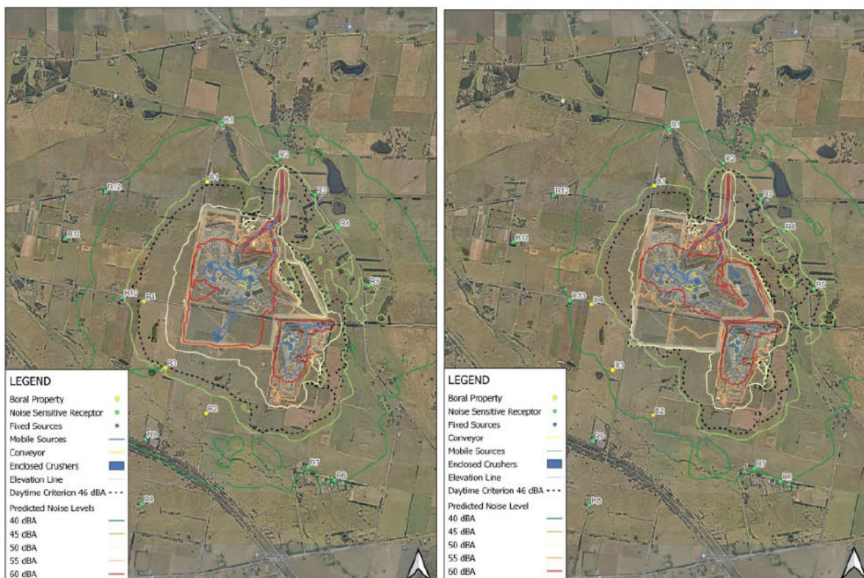
Figure 15 – Excerpts from the Noise Impact Assessment showing noise level contours in relation to surrounding dwellings from the southern pit extension (left) and eastern pit extension (right).
