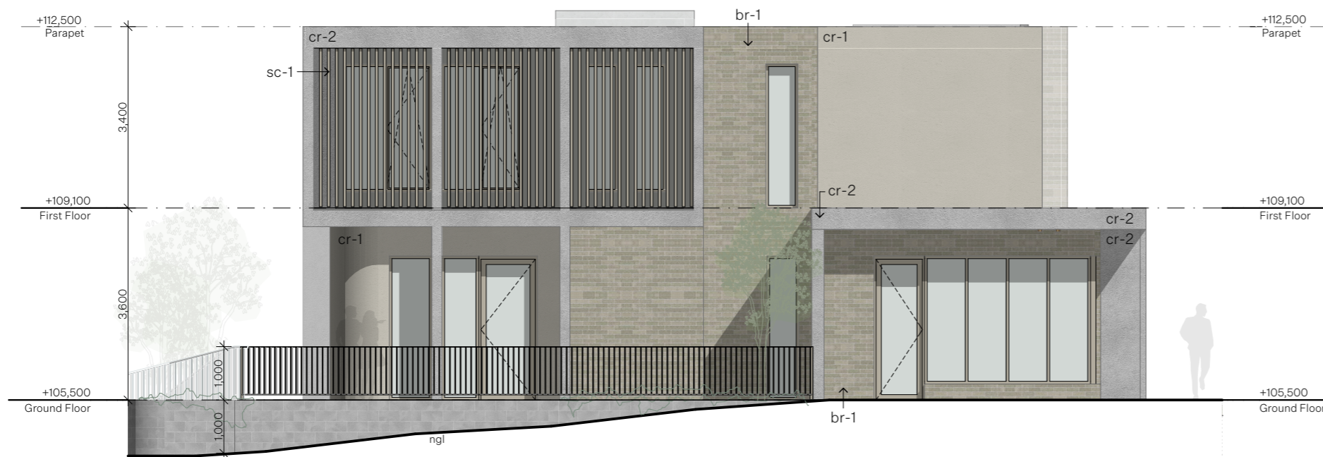
east elevation - water monitoring building
