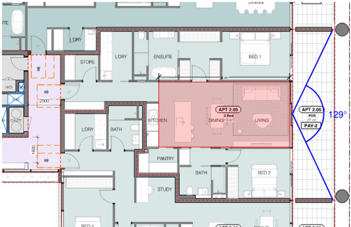
Figure 7. Horizontal Angle of the living room 2.05,3.05,4.05 & 5.05 apartments.
