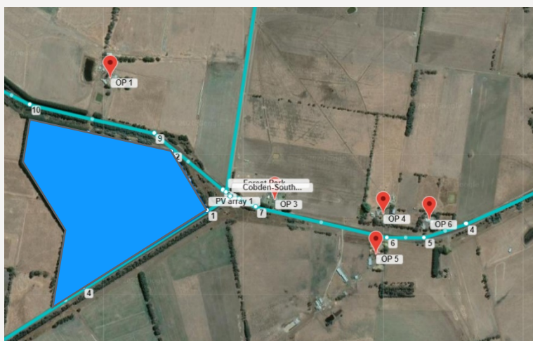
Figure 40 Receptors assessed for glare within the immediate surrounds of the site.
