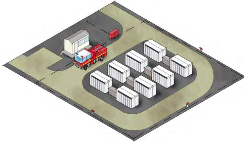
Image 5: Best-practice arrangement of fire service infrastructure for facilities with battery energy storage systems with reticulated water supply meeting the performance requirements of AS 2419.1-2021: Fire hydrant installations (CFA, 2023).
