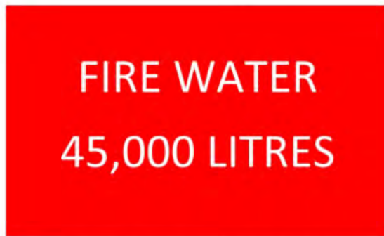
Image 3: Fire water signage to comply with AS 2419.1 Section 5.4.5 (CFA, 2023).
