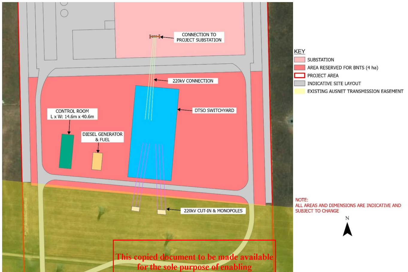
FIGURE 3-3 INDICATIVE PROJECT GRID CONNECTION
