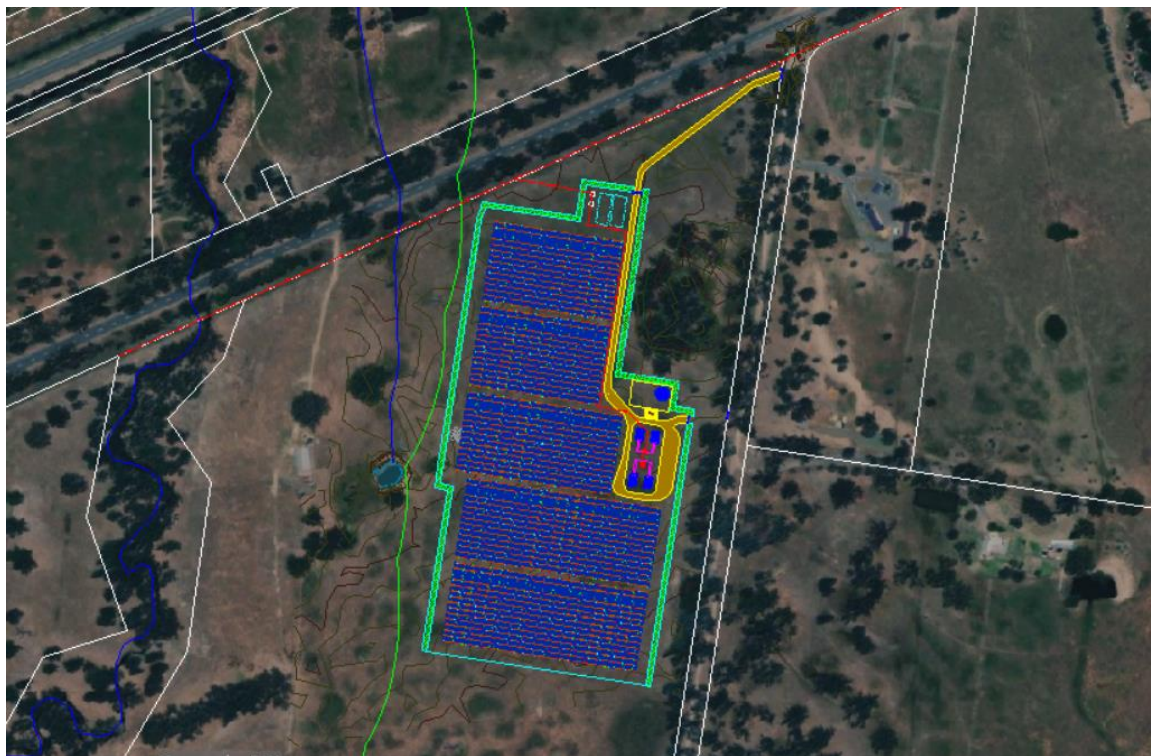
Image 5: Existing design footprint of the PV array using the SMS east-west system.
