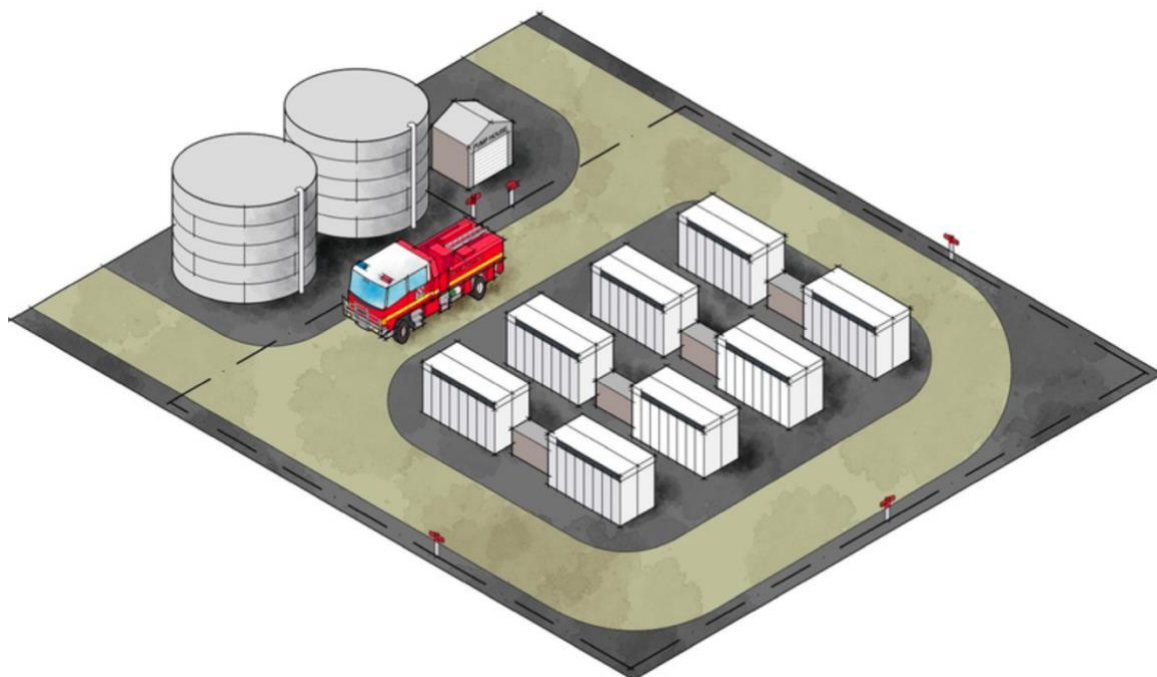
Image 6: Best-practice arrangement of fire service infrastructure at facilities with battery energy storage systems without reticulated water supply, or a reticulated water supply that does not meet the performance requirements of AS 2419.1-2021: Fire hydrant installations (CFA, 2023).
