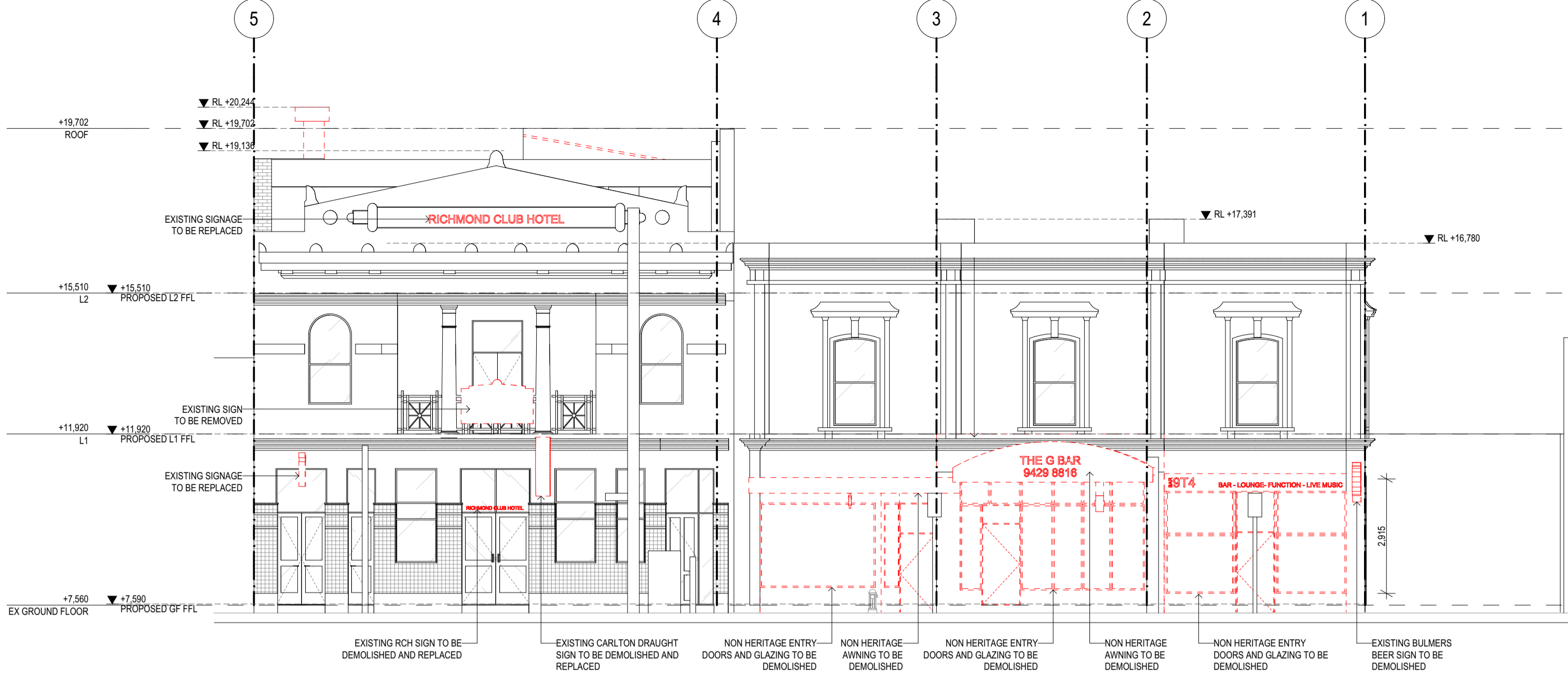
E01 EXISTING/DEMO NORTH ELEVATION (SWAN ST) 1:100
