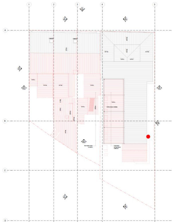
Figure 33 – Ground floor plan showing the extent of demolition to the roof plan.
