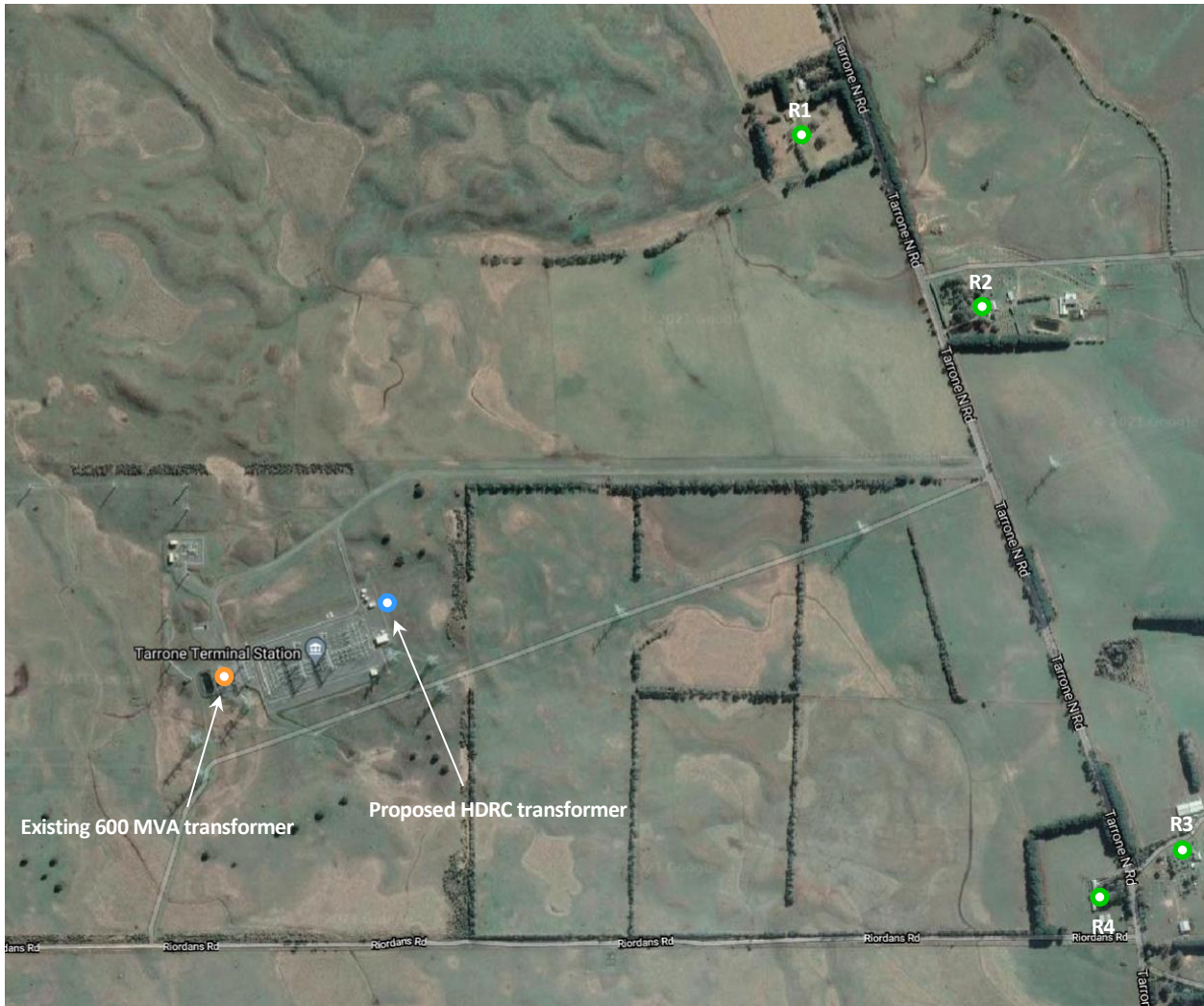
Figure 1: Location map - receivers, existing Macarthur Wind Farm transformer, and proposed HDRC transformer
