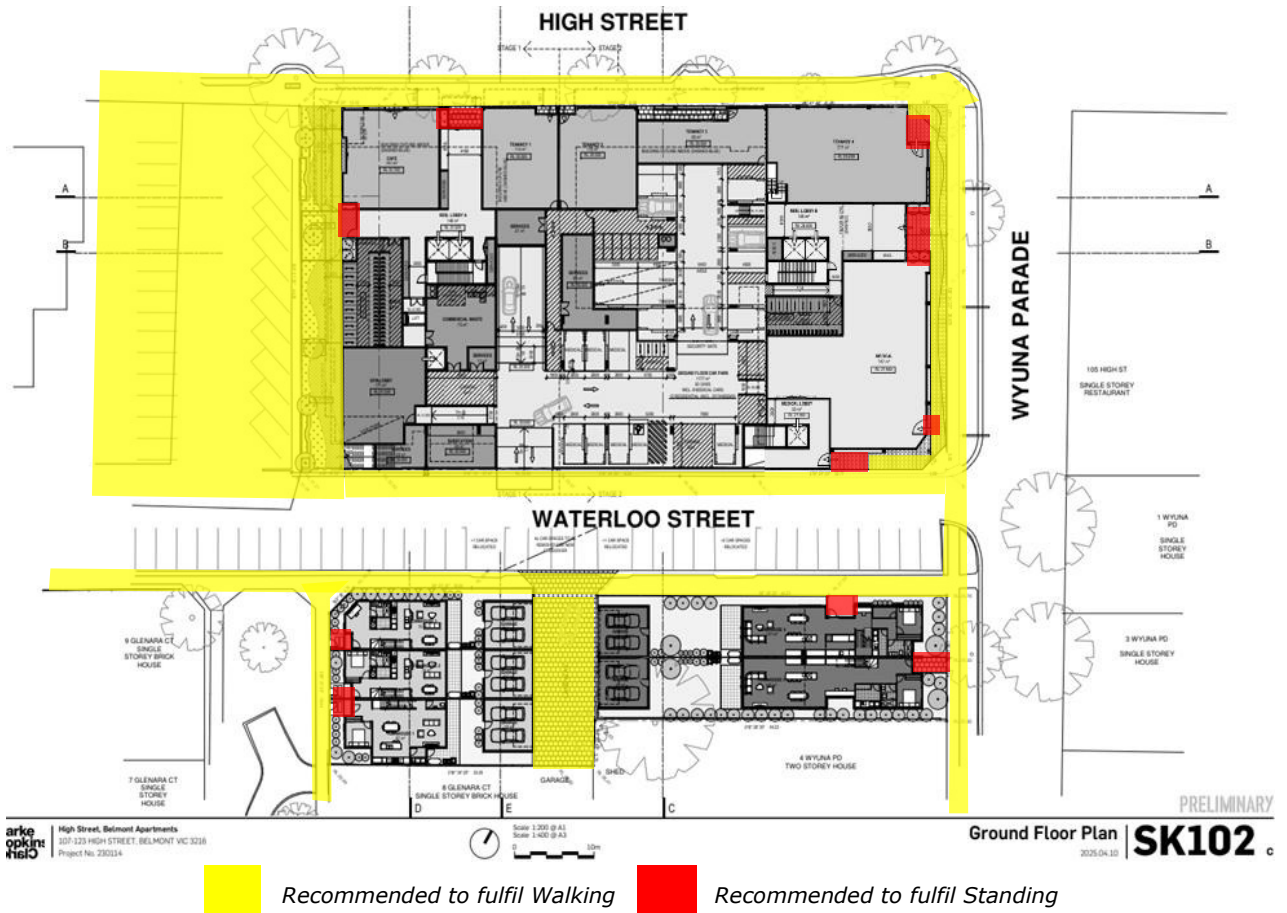
Figure 9: Ground floor plan with recommended wind criteria overlaid.
