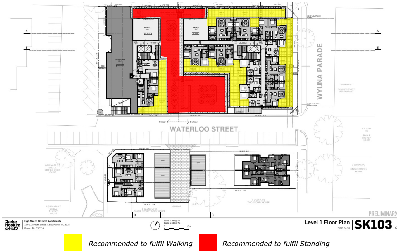
Figure 10: Level 1 plan with recommended wind criteria overlaid
